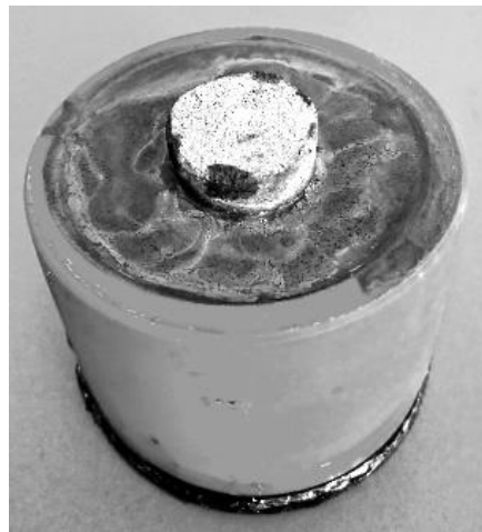
Figure 4. Sample prepared for adhesion tests.
