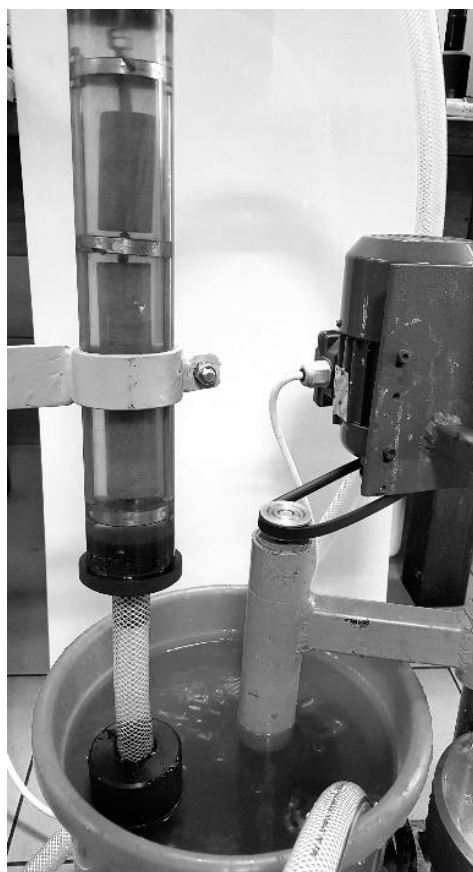
Figure 2. Drilling fluid flow simulator-view of the spacer pumping device.
