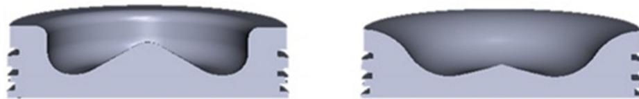
**Figure 11.** Cross-sectional views of the stock (left,) and bathtub (right) piston bowl geometries [43].
