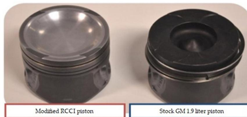
**Figure 16.** A comparison of RCCI and classic CI engines made for dual-fuel research [46].
