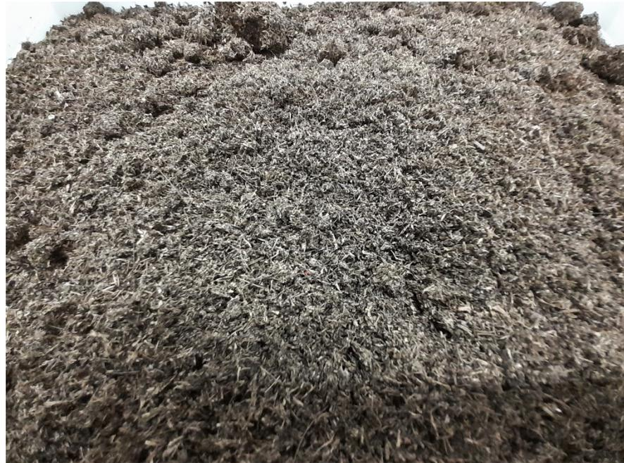
**Figure 2.** Digestate solid fraction.
