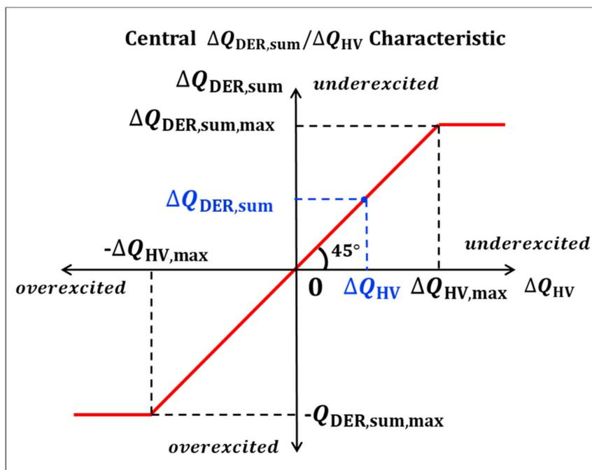
Figure 3. Central  $\Delta Q_{DER,sum}/\Delta Q_{HV}$  PV generation and low load consumption HV curve for Q management at 110 kV-NCP.
