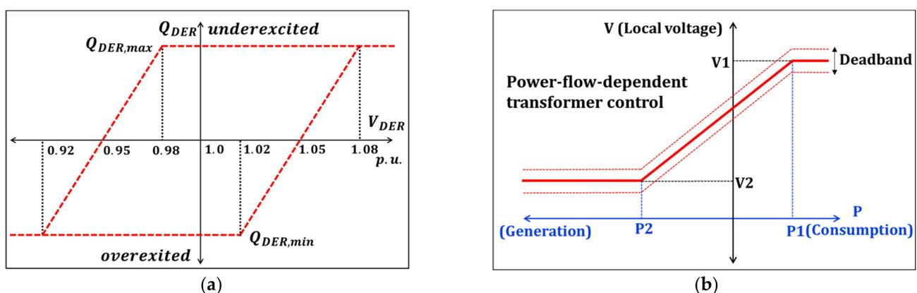
**Figure 7.** The Q(V) limitation characteristic (a) and the applied curve for the power-flow-dependent transformer control (b).
