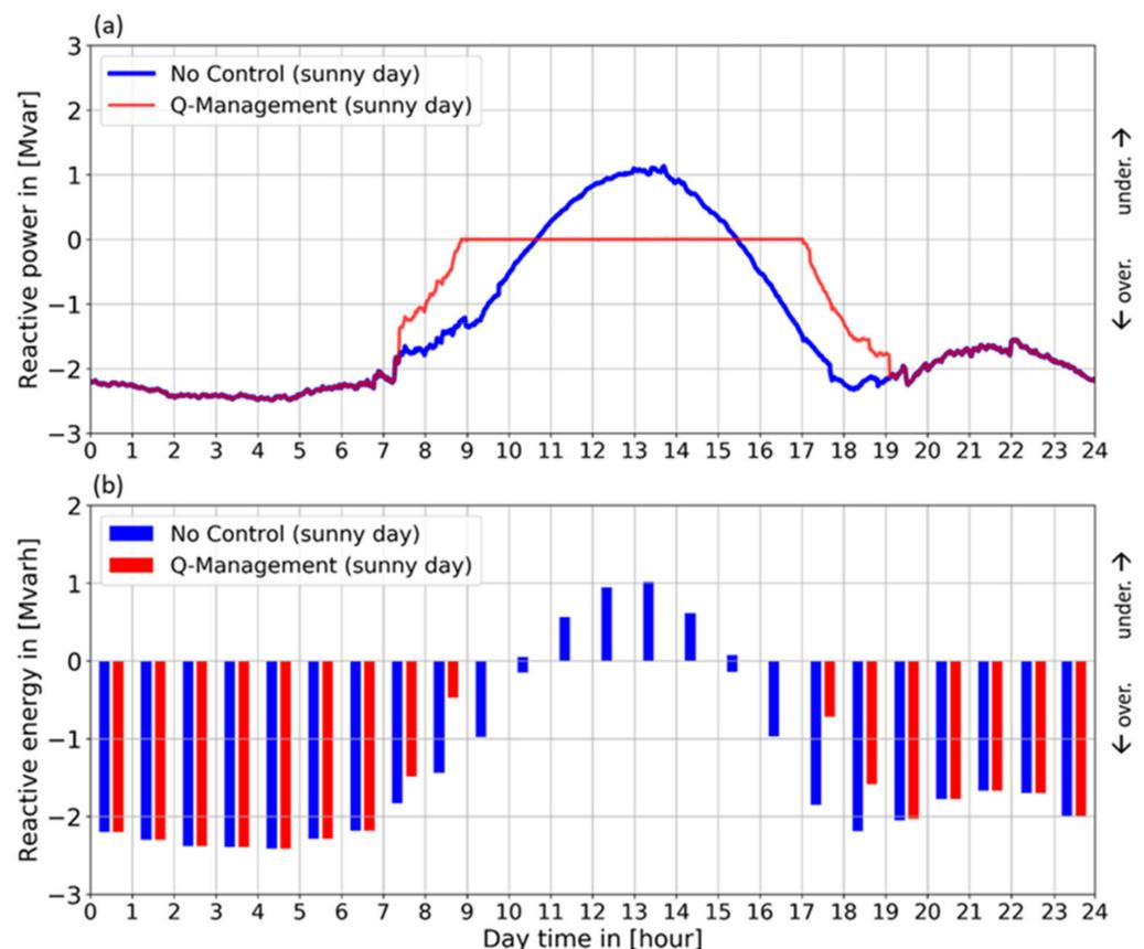
**Figure 8.** Reactive power exchange at 110 kV-NCP (a) and the resulting reactive energy exchange (b) for the investigated sunny summer day (with 1 min control interval).
