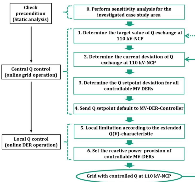
Figure 2. Flowchart of detailed control processes.
