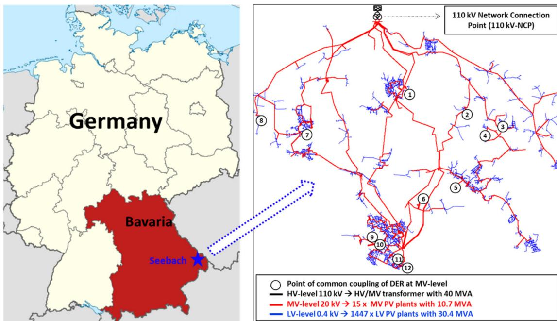
**Figure 6.** The applied multi-voltage-level grid model for the case study area Seebach.
