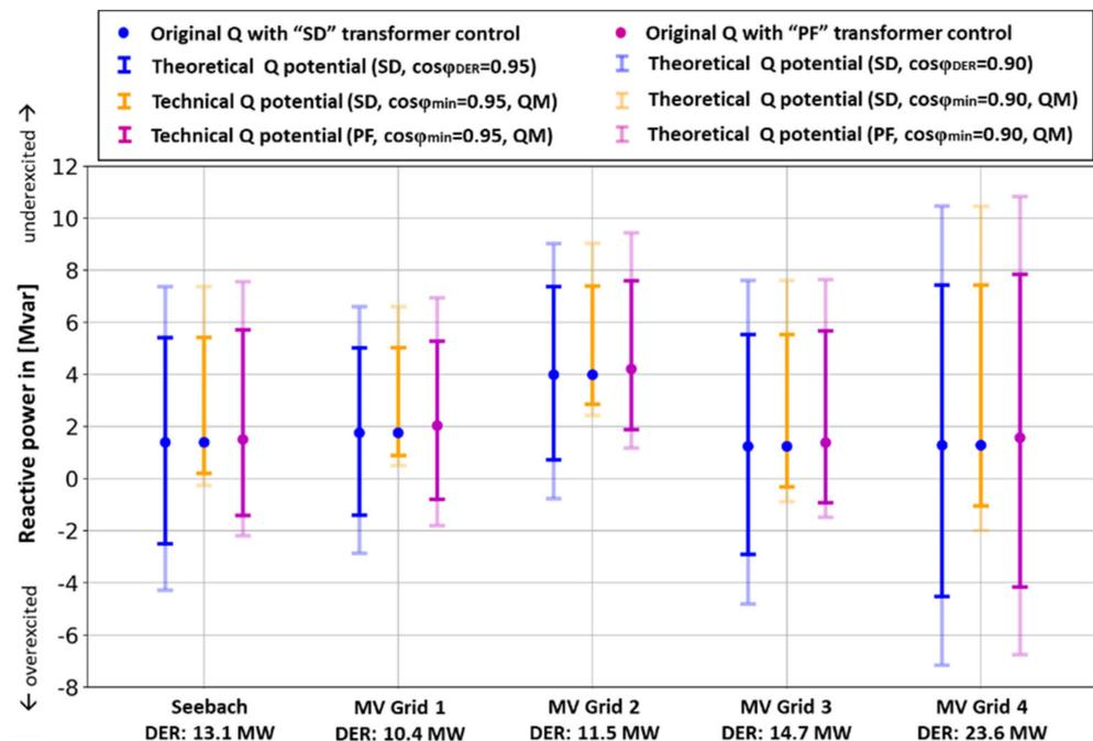
**Figure 14.** Theoretical (blue) and technical potential with standard transformer control (yellow) as well as with power-flow-dependent transformer control (purple) for five different MV grids of Bayernwerk Netz GmbH (in the case of high DER generation and low load consumption).
