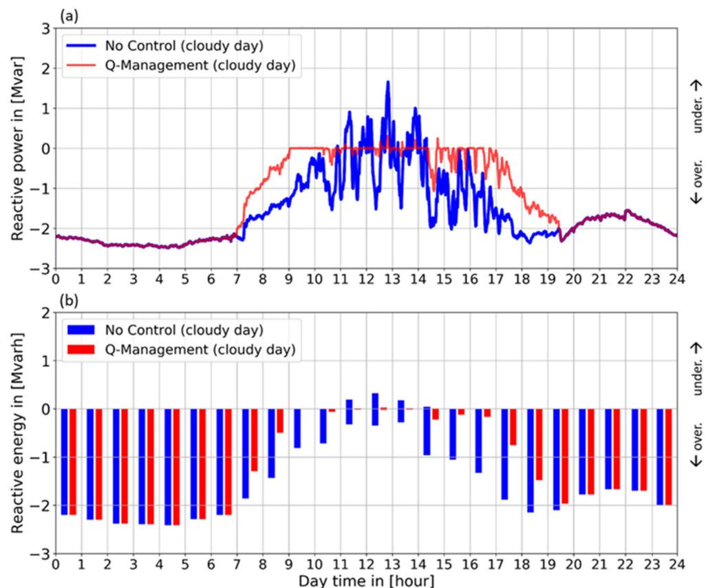
**Figure 9.** Reactive power exchange at 110 kV-NCP (a) and the resulting reactive energy exchange (b) for the investigated cloudy day (with 1 min control interval).
