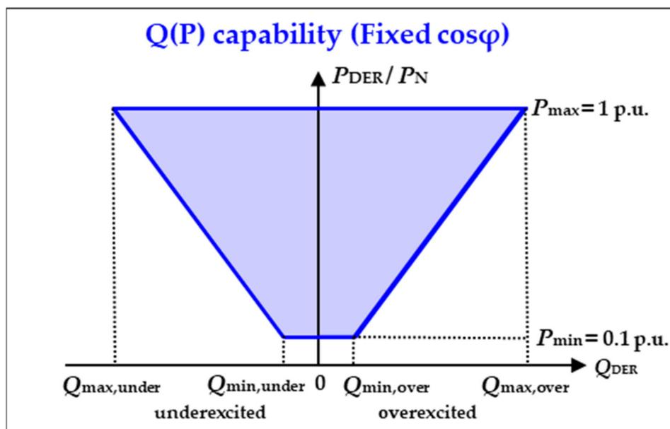
Figure 4. The assumed Q(P) provision capabilities of DERs in this study.
