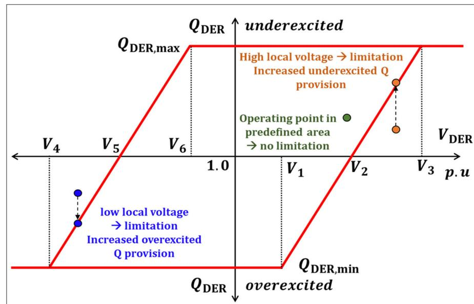
Figure 5. Applied extended Q(V) limitation curve for the voltage limitation.
