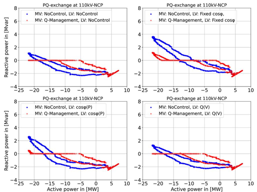
**Figure 13.** Daily simulated P and Q exchange at 110 kV-NCP using the proposed Q management at the MV level and different local voltage control strategies at the LV level.
