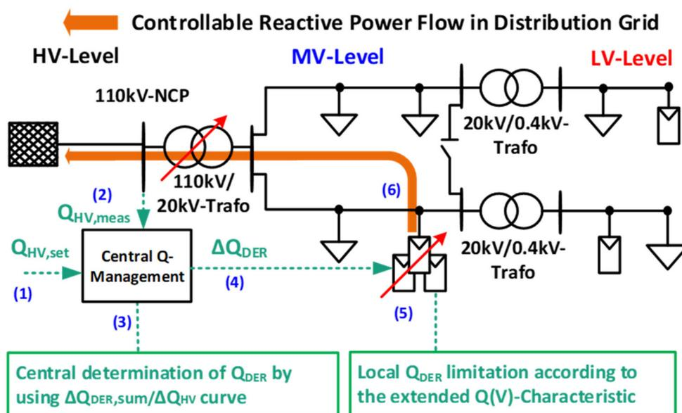
Figure 1. The proposed application-oriented reactive power management concept.
