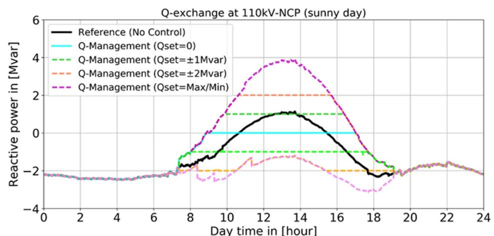
Figure 10. Q exchanges at 110 kV-NCP for simulations with different Q setpoints.
