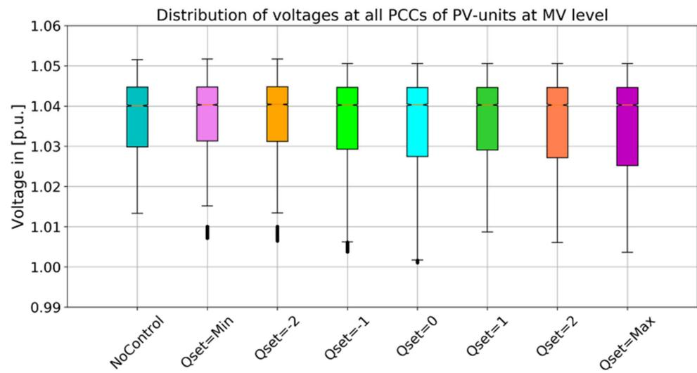
**Figure 11.** Distribution of voltages at PCCs of all controlled PV units with different requested Q setpoints at 110 kV-NCP.
