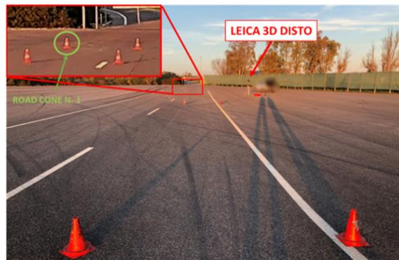
**Figure 20.** Arrangement of road cones on the staked-out points related to vehicle test ruled by the ISO 3888-1 standard and position of the Leica 3D Disto sensor used to measure relative distances.
