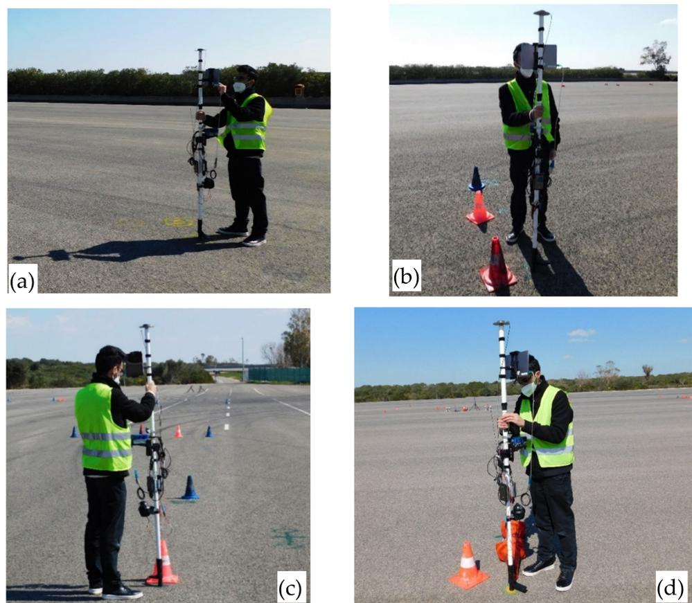
Figure 9. Use of the stake-out geolocation device to locate points with centimeter accuracy on a wide track (a–c) and record geographical coordinates of a point already marked on the ground (d).
