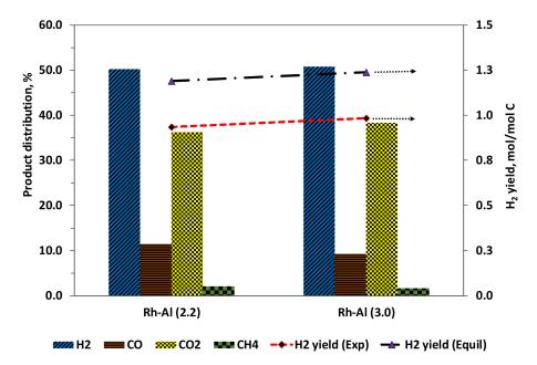
**Figure 15.** Product distribution for bio-oil surrogate ATR using the Rh-Al catalyst at 1 bar and S/C of 2.2 (with 593 °C and  $\lambda$  = 0.318) and S/C of 3 (with 572 °C and  $\lambda$  = 0.391), respectively.
