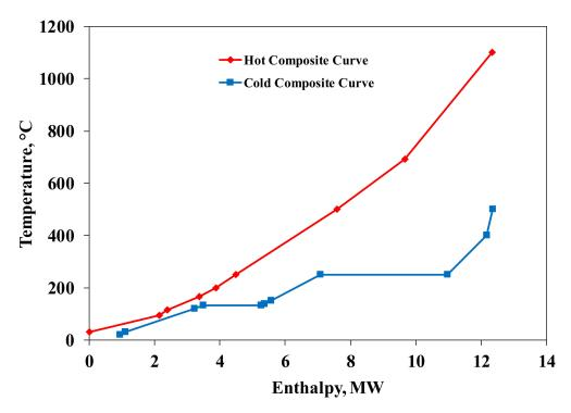
Figure 8. Hot and cold composite curves for base case simulation PAPS process.
