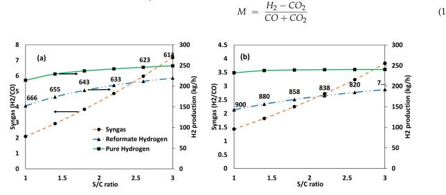
**Figure 5.** Effect of S/C ratio and equivalence ratio  $\lambda$  on syngas ratio H<sub>2</sub>/CO and hydrogen production. For the base case, ATR occur at 3 bar (a)  $\lambda = 0.23$ ; (b)  $\lambda = 0.36$ . Equilibrium temperatures in Celsius degrees (°C) are included as data labels.
