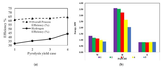
**Figure 10.** (a) Influence of pyrolysis product yield on the overall process efficiency and the hydrogen efficiency. The five cases examined are labelled from 1 to 5 in order of increasing bio-oil yield. (b) Turbine work output 'W', heat output 'H' and electrical input 'E' for the various pyrolysis yield cases examined in this study.
