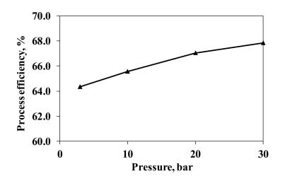
**Figure 11.** Influence of pressure on overall process efficiency for a 5000 kg/h PEFB plant operating at 3, 10, 20 and 30 bar.
