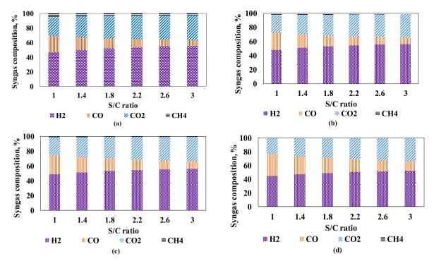
**Figure 4.** Syngas yield on a dry nitrogen-free basis. For the base case, ATR and shifting occur at 3 bar and H<sub>2</sub> recovery is carried out at 10 bar (a)  $\lambda = 0.23$ ; (b)  $\lambda = 0.25$ ; (c)  $\lambda = 0.28$ ; (d)  $\lambda = 0.36$ .
