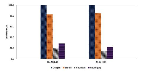
**Figure 14.** Conversion of oxygen, bio-oil, and water (experiment and equilibrium) using Rh-Al catalyst at 1 bar with reactor bed temperatures of 593 °C ( $\lambda$  = 0.318) and 572 °C ( $\lambda$  = 0.391) for S/C ratios of 2.2 and 3, respectively (S/C ratio in brackets next to catalyst name).
