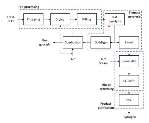
Figure 1. Process flow diagram for hydrogen production from 40 wt.% moist PEFB biomass.
