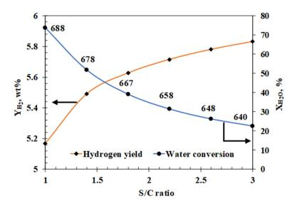
**Figure 3.** Influence of the amount of steam, expressed as S/C ratio, on hydrogen yield for equivalence ratio,  $\lambda = 0.25$ . For the base case, ATR and CO-shift occur at 3 bar and H<sub>2</sub> recovery is carried out at 10 bar. Equilibrium temperatures in Celsius degrees (°C) are included as data labels.
