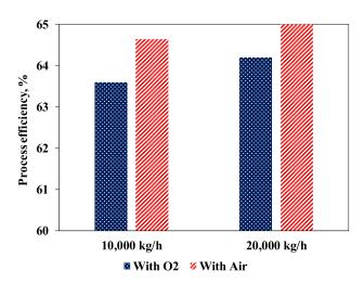
**Figure 12.** Overall process efficiencies for systems using air and systems using oxygen. (left) 10,000 kg/h PEFB plant, (right) 20,000 kg/h PEFB plant.
