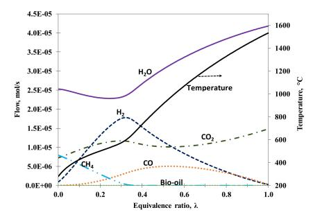
**Figure 13.** Thermodynamic equilibrium plots showing syngas composition and temperature obtained at S/C = 2.2 and 1 bar while varying  $\lambda$  from 0 to 1 for bio-oil surrogate (m.f.) ATR.
