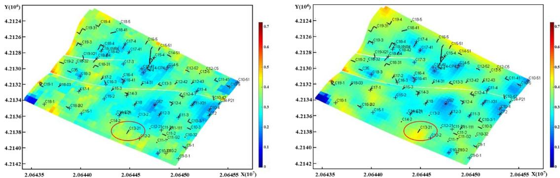
Figure 11. The average remaining oil saturation distribution (the left one is calculated by a traditional simulator, the right one is calculated by the new simulator).
