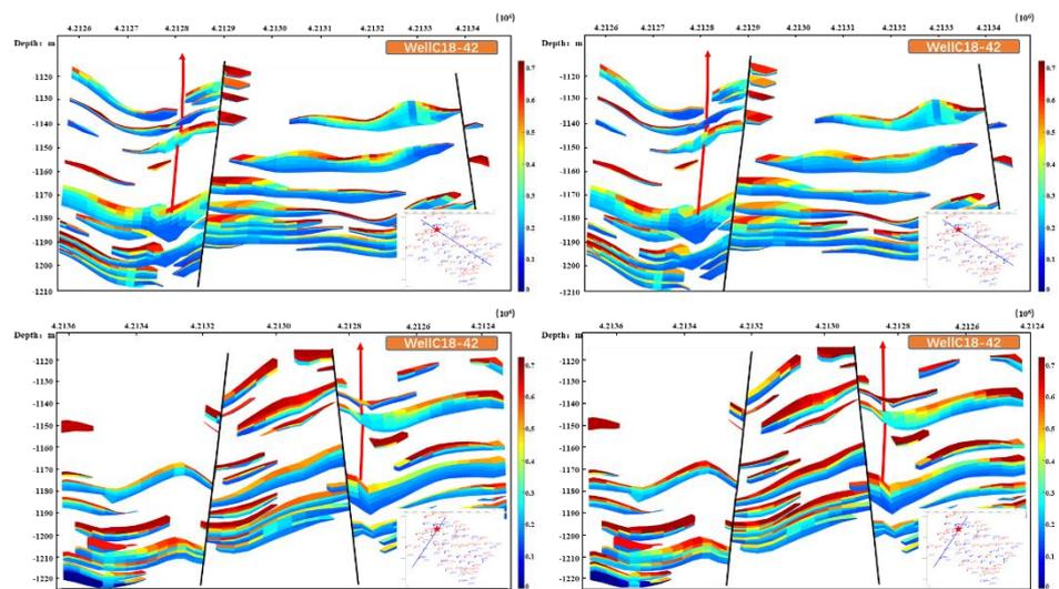
**Figure 13.** Cross section of remaining oil saturation of well C18-42 (the upper left one and the lower left one are the remaining oil profiles calculated by the numerical simulation method considering anisotropic relative permeability, and the upper right one and lower right one are the results of a traditional simulation).
