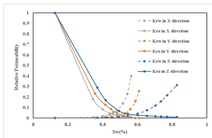
**Figure 3.** Relative permeability of three directions.
