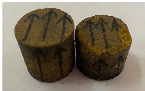
Figure 8. Photo of palaeomagnetic core sample.
