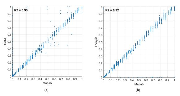
**Figure 19.** Scatter plots for the direct irradiance shading factor  $f_B$ . Comparison of: (a) Matlab with SAM and (b) Matlab with PVsyst. Results are for situation 1, one module shaded by a single obstacle positioned on the east side.
