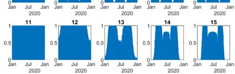
**Figure 26.** Direct shading factor  $f_B$  as a function of time for all the modules in the array.
