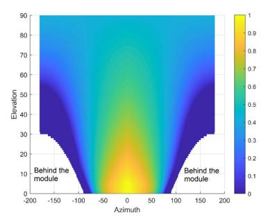
**Figure 9.** Heat map representation of the shading table. Yellow portions correspond to higher shading factors for the direct irradiance. Blue values correspond to low shading factors for the direct irradiance. The white parts on the bottom left and right corners of the heat map correspond to angles where the sun is behind the module (NaN values).
