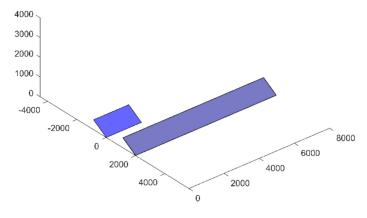
**Figure 12.** First module of the second row being shaded by the row in front. The shading factor for the inter-row shading is calculated for each module of the second row, being shaded by an obstacle with the size of the row in front.
