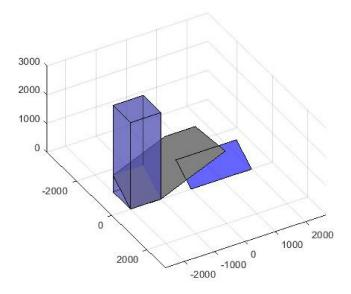
**Figure 7.** Visual output of one module and one obstacle casting a shadow on the plane defined by the module.
