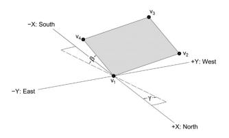
**Figure 2.** Geometric definition of the vertices  $v_1$ ,  $v_2$ ,  $v_3$ , and  $v_4$  for a solar module with tilt angle  $\beta$  and azimuth angle  $\gamma$ . Azimuth angles are measured from north and positive clockwise.
