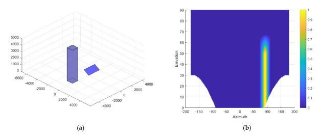
**Figure 13.** Situation 1, one PV module being shaded by one obstacle positioned on its east side with 2 m of separation. The tilt angle of the module is  $30^{\circ}$  and the azimuth angle is  $0^{\circ}$ : (a) Visual output; (b) Heat plot representation of the shading table.
