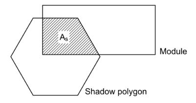
**Figure 8.** Area of the shadow that falls on the surface of the module. The previously calculated shadow polygon must be cropped in order to find the portion of shadow that falls on the module  $(A_s, hatched area)$ .
