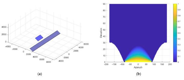
**Figure 14.** Situation 2, one PV module being shaded by one infinite row in front. The tilt angle of the row is  $30^{\circ}$  and is positioned at 2 m from the module. The tilt angle of the module is  $30^{\circ}$  and the azimuth angle is  $0^{\circ}$ : (a) Visual output; (b) Heat plot representation of the shading table.
