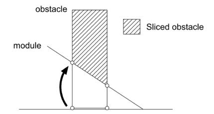
**Figure 5.** Side view of one module and one obstacle. If some of the obstacle vertices are behind the module plane, it is possible to slice the obstacle by moving these vertices vertically until they are positioned on the plane.
