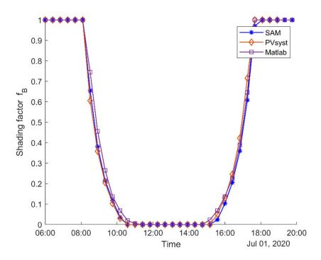
**Figure 16.** Shading factor  $f_B$  for situation 2 calculated for one day (1 July).  $f_B$  was calculated with the System Advisor Model (SAM), PVsyst, and the proposed Matlab tool.
