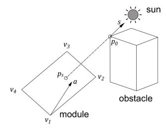
**Figure 4.** A vertex  $p_0$  of one obstacle is projected on the plane defined by the module. The projected point is called  $p_s$ . The vector *s* is a vector pointing towards the sun. The vector *a* is normal to the plane of the module.  $v_1$ ,  $v_2$ ,  $v_3$ , and  $v_4$  are the positions of the vertices that define the module.
