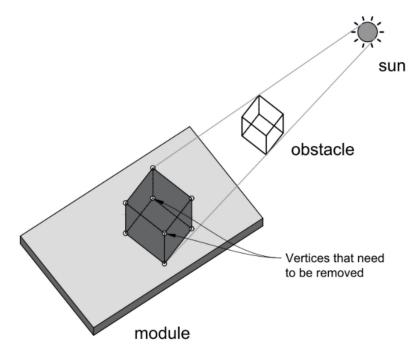
**Figure 6.** Projection of each of the eight obstacle vertices onto the surface of the module. After projecting all the points, there are two points that need to be removed. These two points are internal to the shadow and do not correspond to the ones located on the perimeter of the shadow.
