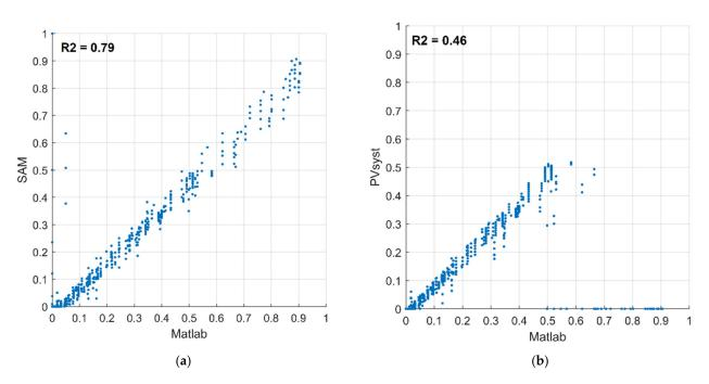
**Figure 20.** Scatter plots for the direct irradiance shading factor  $f_B$ . Comparison of: (a) Matlab with SAM and (b) Matlab with PVsyst. Results are for situation 2, one module shaded by one infinite row.
