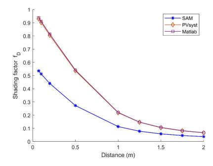
**Figure 23.** Diffuse shading factor for a module shaded by an infinite row, assuming different distances of separation.
