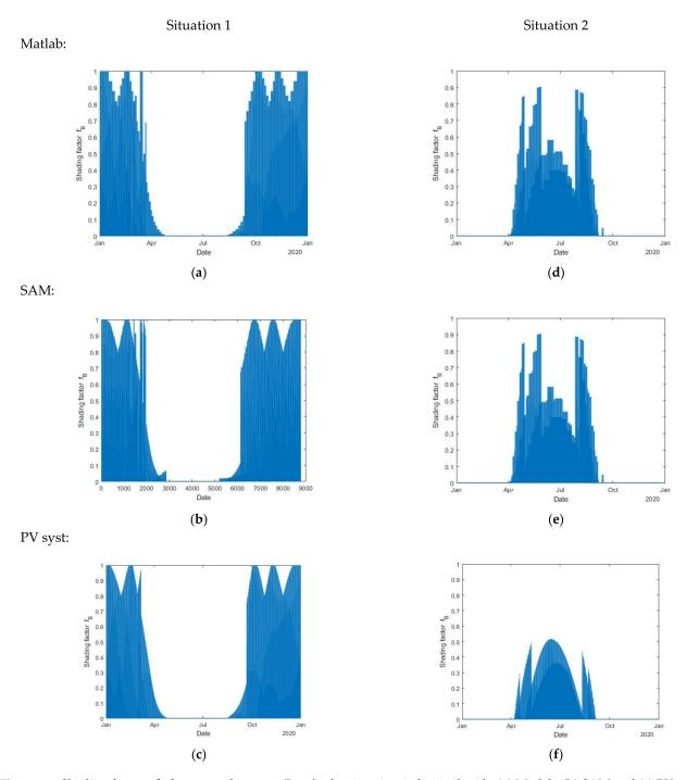
**Figure 18.** Shading factors  $f_B$  for a complete year. Results for situation 1 obtained with: (a) Matlab; (b) SAM and (c) PVsyst. Results for situation 2 obtained with (d) Matlab; (e) SAM and (f) PVsyst.
