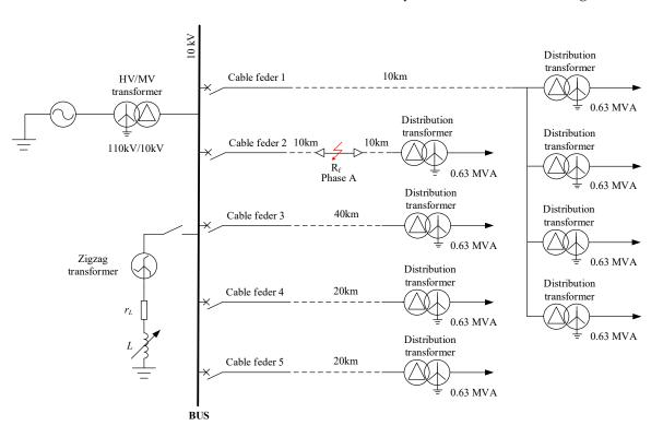
Figure 8. Simulation model of the resonant grounded distribution.
