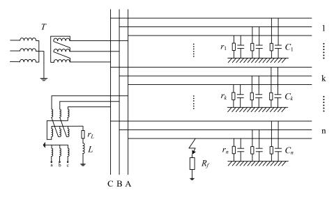
**Figure 1.** A phase-to-ground fault in the resonant grounded distribution system, where *T* is the HV/MV transformer, and  $R_f$  is the fault resistance. *C* is the equivalent capacitance of the system. *r* is the equivalent resistance of the system. *L* is the equivalent inductance of the arc suppression coil.  $r_L$  is the equivalent inductance of the arc suppression coil.
