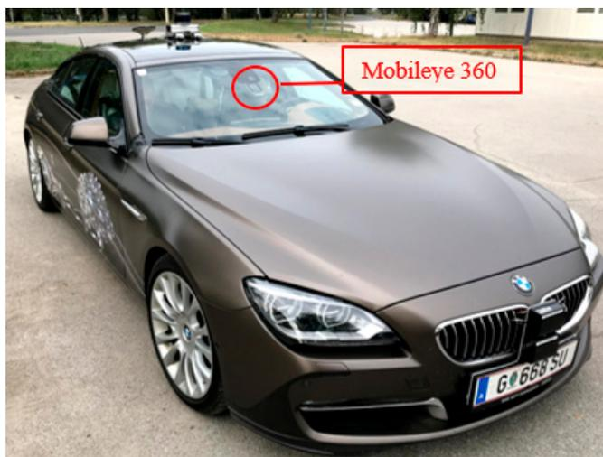
**Figure 1.** Testing vehicle with Mobileye 360 implemented behind the front windshield inside the vehicle.
