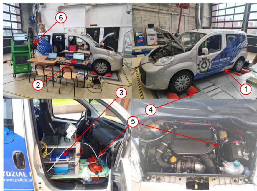
**Figure 1.** Test stand consisting of: 1. Fiat Qubo test car with 1.3 Multijet engine; 2. computer with installed AVL Indicom V2.7 software; 3. Indimicro 602 engine indicator system; 4. DF4FS-HLS chassis dynamometer; 5. additional fuel system tank; 6. KTS Bosch diagnostic module.
