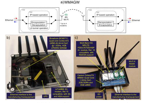
**Figure 4.** (a) Functional block diagram of the WMAGWs (operating in device-to-device L2-tunnel mode). Note: for IP-based operation, the alternative path is chosen via SW configuration. Infrastructure mode is supported by using the exam same functional blocks. (b) Picture of the implemented WMAGW prototype (v2) including details on the different HW components. (c) Picture of the implemented WMAGW prototype (v3) including details on the different HW components.
