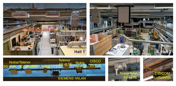
**Figure 2.** Overview of the Aalborg University 5G Smart Production Lab, including details on the two industrial halls and the different operational wireless network deployments.
