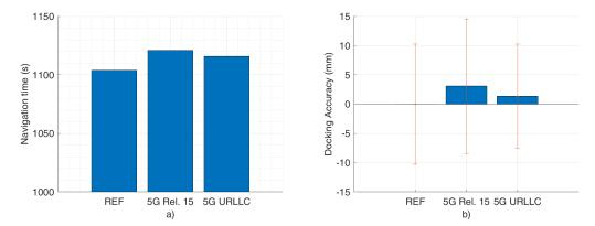
docking accuracy test, the results are shown in Figure 12b, and they illustrate that the use of the 5G MEC planner would result in a slight loss of accuracy of maximum 1–3 mm, which would be negligible for reliable operation of the AMRs.
