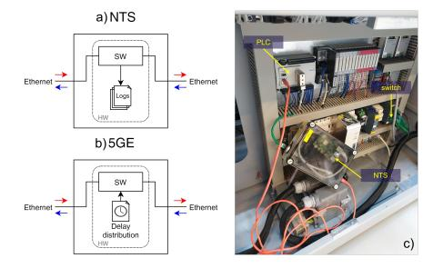
**Figure 3.** (a) Functional block diagram of the NTS. (b) Functional block diagram of the 5GE. (c) Picture of the NTS/5GE (v2) device deployed within a production line module. Under such exact same deployment configuration, the box can be used to either logging the data traffic to and from a PLC, or to introduce communication delays to emulate the connectivity of the PLC over 5G wireless.
