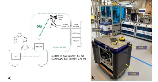
**Figure 11.** (a) Architecture of the 5G-integrated MEC AMR planner solution including the AMR, WMAGW, 5G network infrastructure, and AMR fleet manager controller and planner deployed in edge-cloud configuration. (b) Picture of the 5G-integrated MEC AMR planner solution deployed for 5G emulation at the lab.
