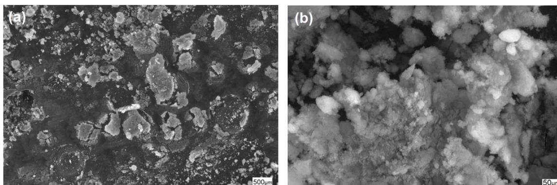
**Figure 2.** SEM images of the silica/lignin carrier at different magnifications: (a) 500 μm and (b) 50 μm diameter particles.
