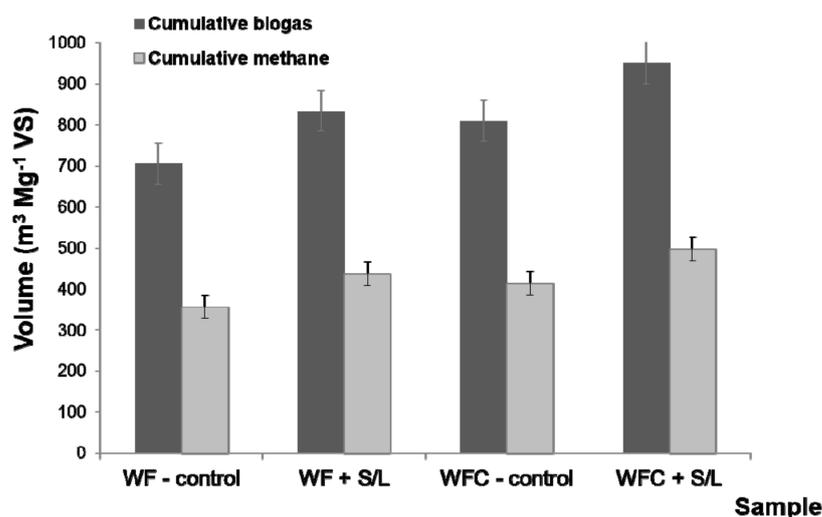
**Figure 6.** Cumulative biogas and methane yield from tested samples.
