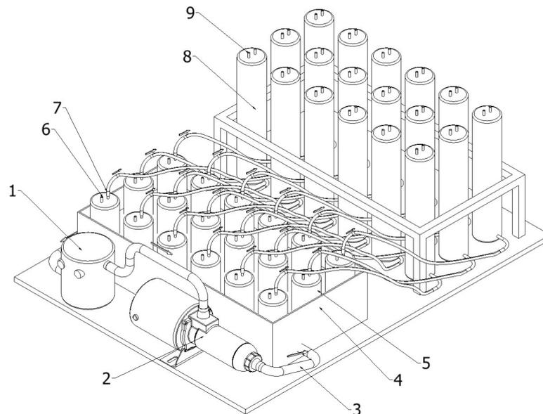
**Figure 1.** The (12-chamber) anaerobic bioreactor that was employed for the biogas production experiment: 1-water heater; 2-water pump; 3-insulated heating tubes; 4-water jacket (39 °C); 5-bioreactor (1.4 L); 6-slurry sampling valve; 7-biogas transport tube; 8-graduated biogas tank; 9-gas sampling valve.
