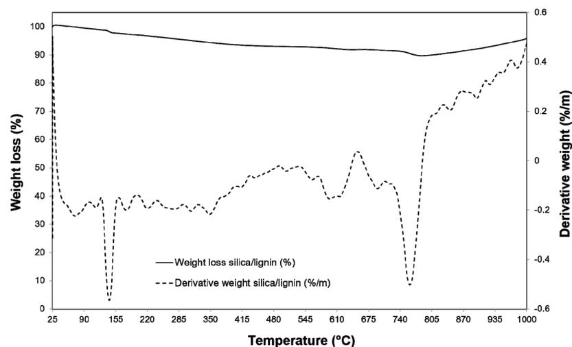
**Figure 4.** Thermograms of the silica/lignin carrier.
