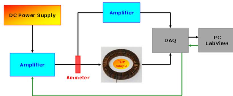
Figure 5. Magnetic characterization system setup with Lab View platform (DAQ—Data Acquisition).
