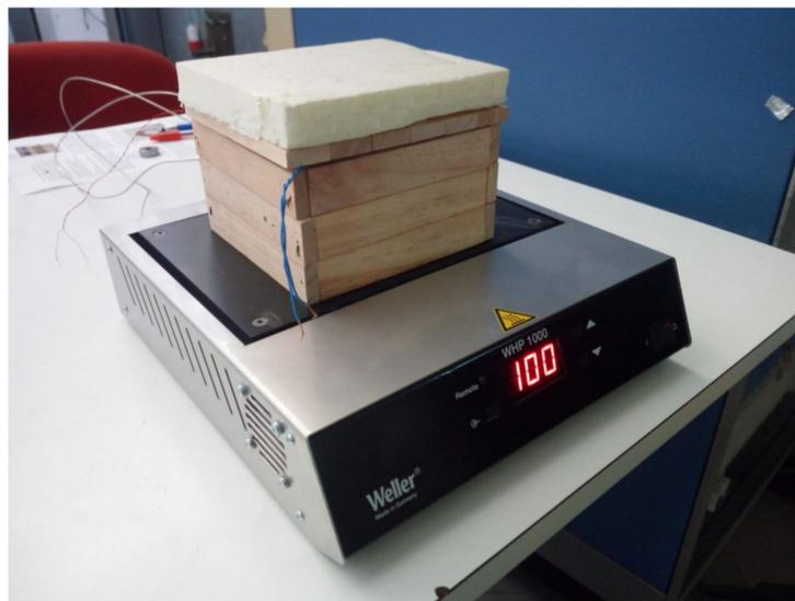
**Figure 2.** The heating process: chamber and heater at 100 °C.
