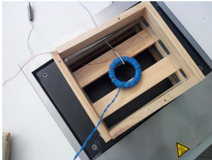
**Figure 1.** The toroid Soft Magnetic Composite (SMC) samples inside the implemented chamber (without cover).
