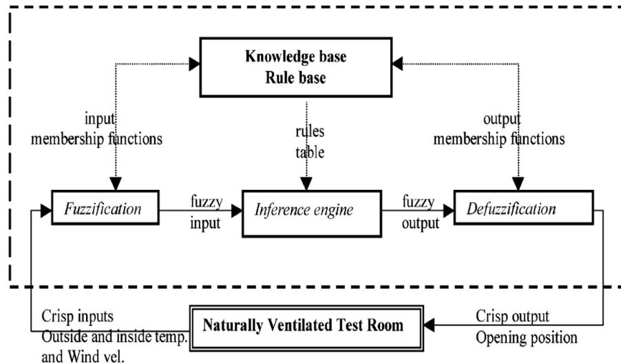
Figure 3. Basic configuration of fuzzy logic controller [57].
