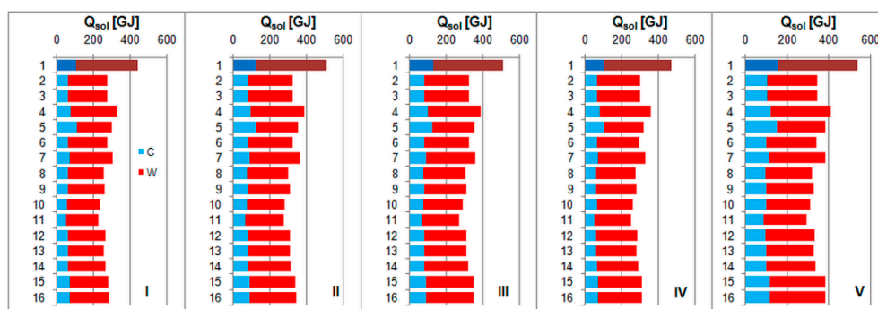
Figure 8. Total annual solar heat gains for Building 2, Variant 1.
