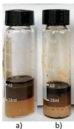
Figure 1. Results of phase behavior study for (a) EW-surfactant solution and (b) EW-surfactant solution with addition of 1 wt% alkali.
