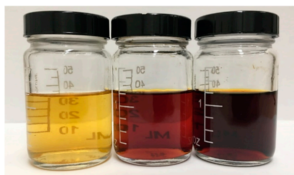
Figure 7. Filtered liquid smokes from light to severe microwave torrefaction (left to right).
