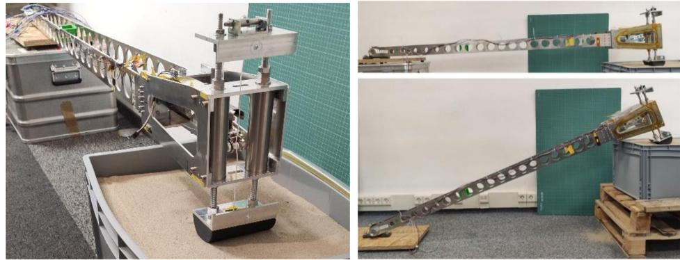
**Figure 6.** (Left) The actual implementation of the compression springs suspension in the BB-0B testbed. (Right) Horizontal ( $0^\circ$ ) and inclined ( $20^\circ$ ) configurations of the testbed.
