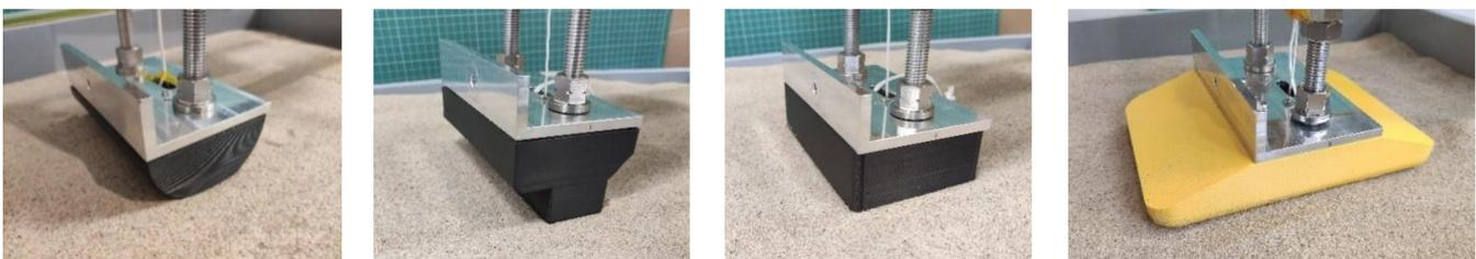
**Figure 12.** From left: configuration #1 with a cylindrical 3D-printed foot in contact with quartz sand; configuration #2 actuating leg with a flat surface contact area same as config #1; configuration #3 with a flat surface contact area based on a width equivalent to the diameter of the round foot; configuration #4 with a flat foot with a contact area 4.8 times greater than contact area from the configuration #1 and #2.
