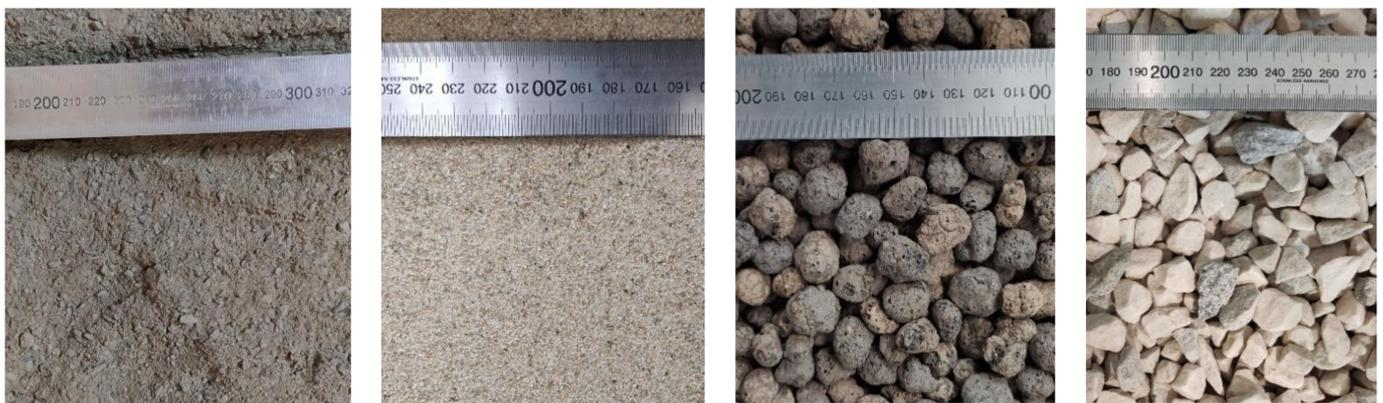
**Figure 14.** The type of surface materials used in the tests. From left: Syar, quartz sand, expanded clay, quartz aggregate.
