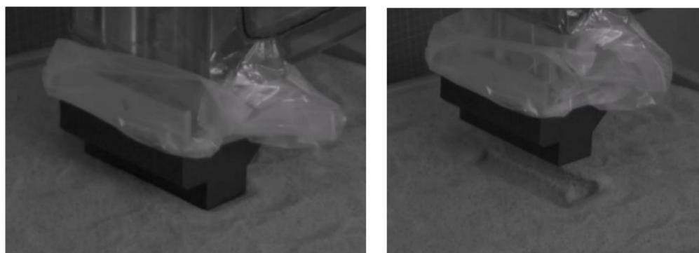
**Figure 19.** Jump in quartz sand with the foot in configuration #2.
