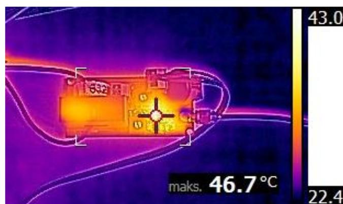
**Figure 11.** IR photo of the proposed sensor in steady state operation under a full load current (40 A).
