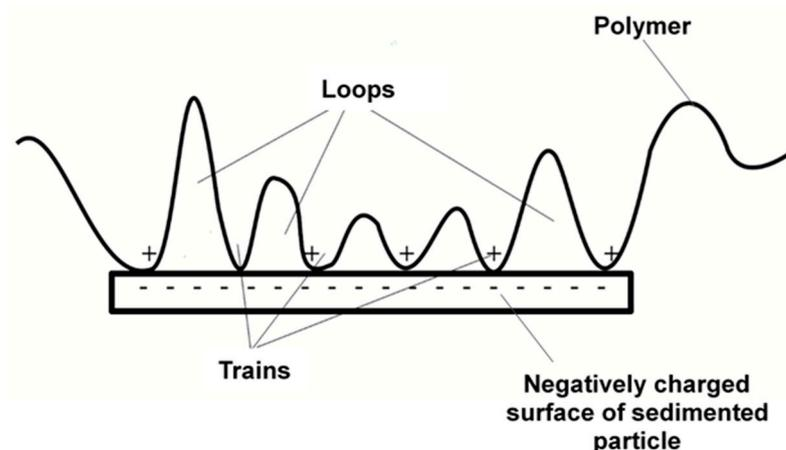
**Figure 3.** Polymer adsorption on surface of solid particle.
