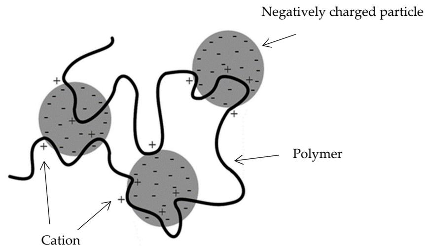
**Figure 4.** Mechanism of bridging flocculation.
