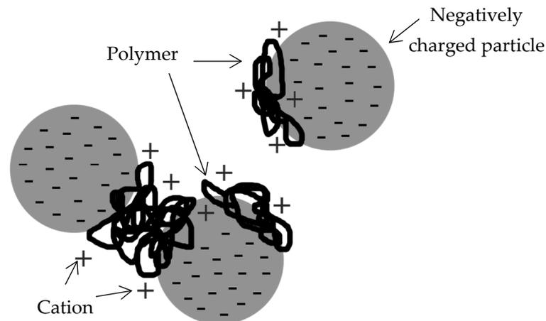
**Figure 2.** Mechanism of patching flocculation.
