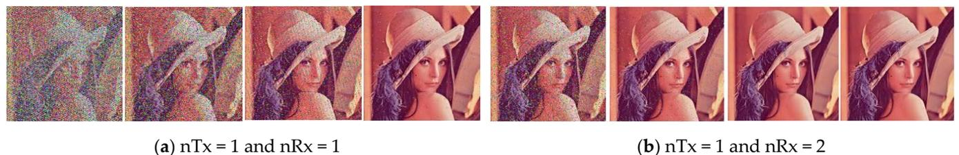
**Figure 5.** Received Image with DCT-OFDM over a AWGN channel, Modulated with QPSK and at SNR = 0, 5, 10, 15 dB from  $L \Rightarrow R$  with MRC ( $n_{Tx} = 1$  and  $n_{Rx} = 1$  and 2).
