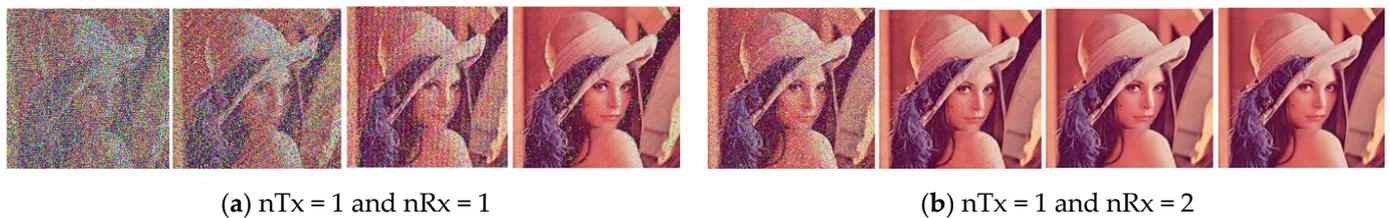
**Figure 4.** Received Image with FFT-OFDM over a AWGN channel, Modulated with QPSK and at SNR = 0, 5, 10, 15 dB from  $L \Rightarrow R$  with MRC ( $n_{Tx} = 1$  and  $n_{Rx} = 1$  and 2).
