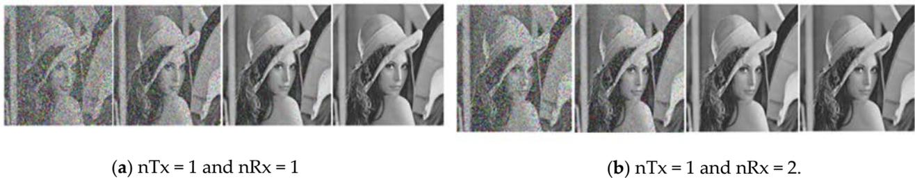
**Figure 11.** Received Image with DCT-OFDM over a Rayleigh channel, Modulated with QPSK at  $E_b/N_0 = 0, 5, 10, 15$  dB from left to right with MRC ( $n_{Tx} = 1$  and  $n_{Rx} = 1$  and 2).
