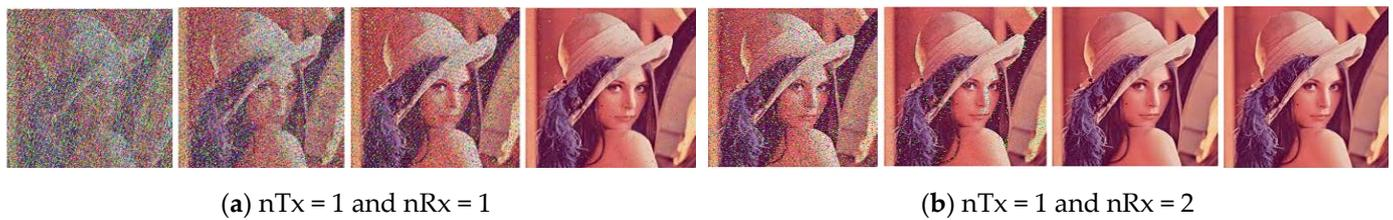
**Figure 7.** Received Image with DCT-OFDM over a Rayleigh channel, Modulated with QPSK and at SNR = 0, 5, 10, 15 dB from L => R with MRC ( $n_{Tx} = 1$  and  $n_{Rx} = 1$  and 2).
