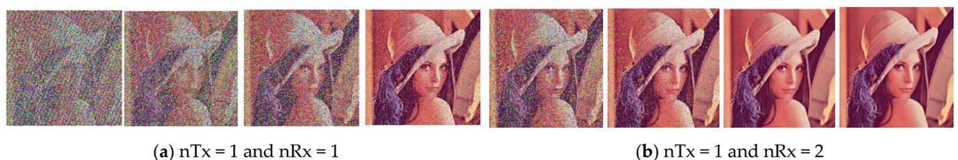
**Figure 6.** Received Image with FFT-OFDM over a Rayleigh channel, Modulated with QPSK and at SNR = 0, 5, 10, 15 dB from  $L \Rightarrow R$  with MRC ( $n_{Tx} = 1$  and  $n_{Rx} = 1$  and 2).
