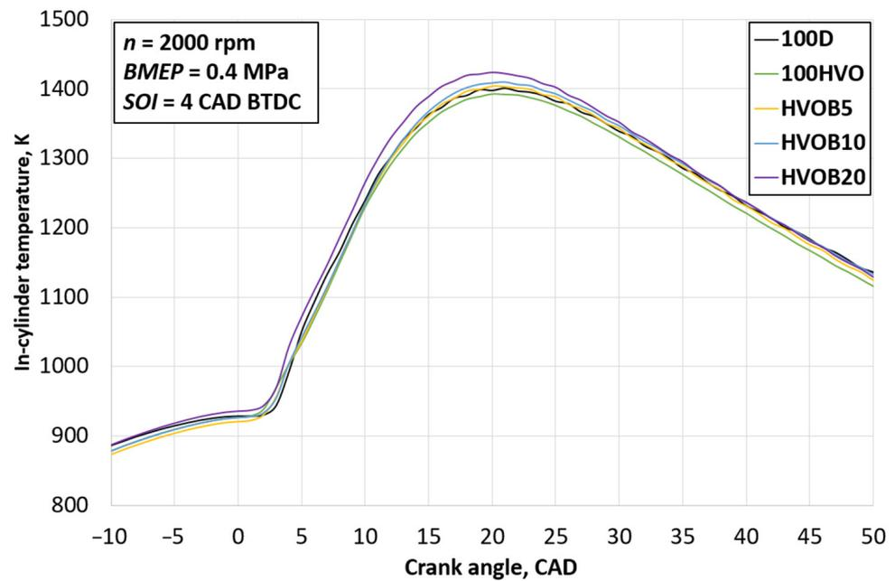
Figure 6. In-cylinder temperature depending on fuel composition.
