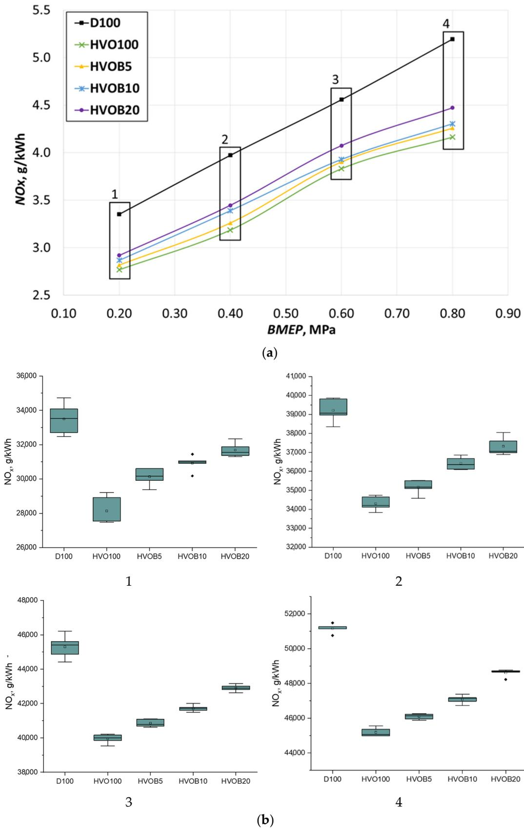
**Figure 18.** Dependence of NO<sub>x</sub> emission on fuel composition and the engine load: (a) summary of results; (b) accuracy and errors of measurements.
