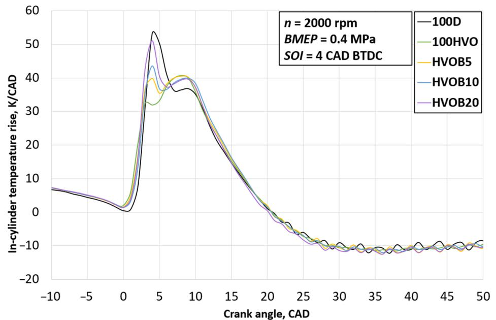
Figure 5. Temperature rise in-cylinder depending on fuel composition.
