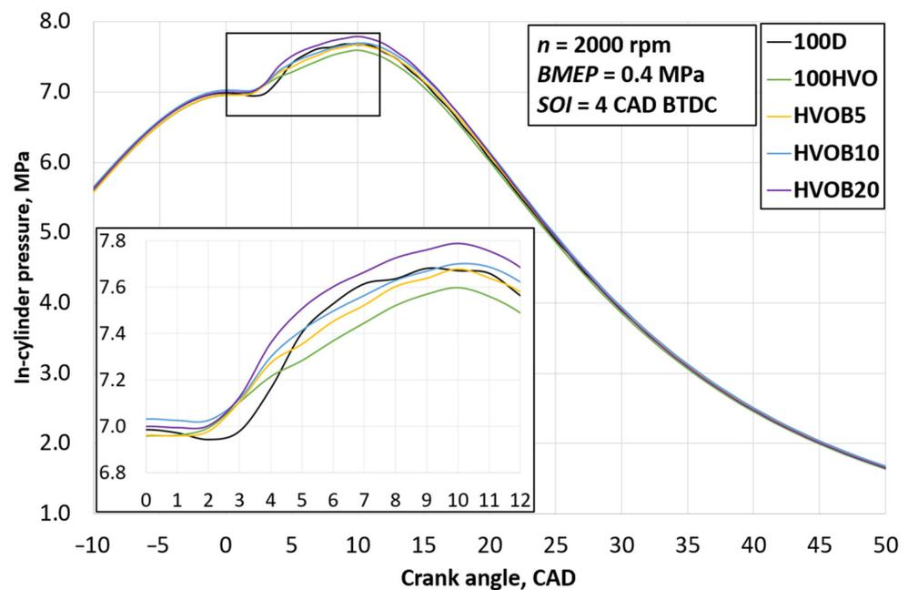
**Figure 8.** In-cylinder pressure depending on fuel composition.
