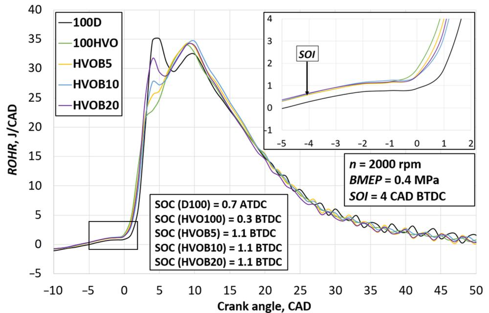
Figure 4. Rate of heat release in-cylinder depending on fuel composition.
