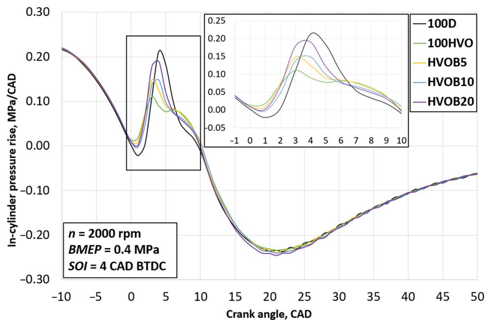
Figure 7. Pressure rise in-cylinder depending on fuel composition.
