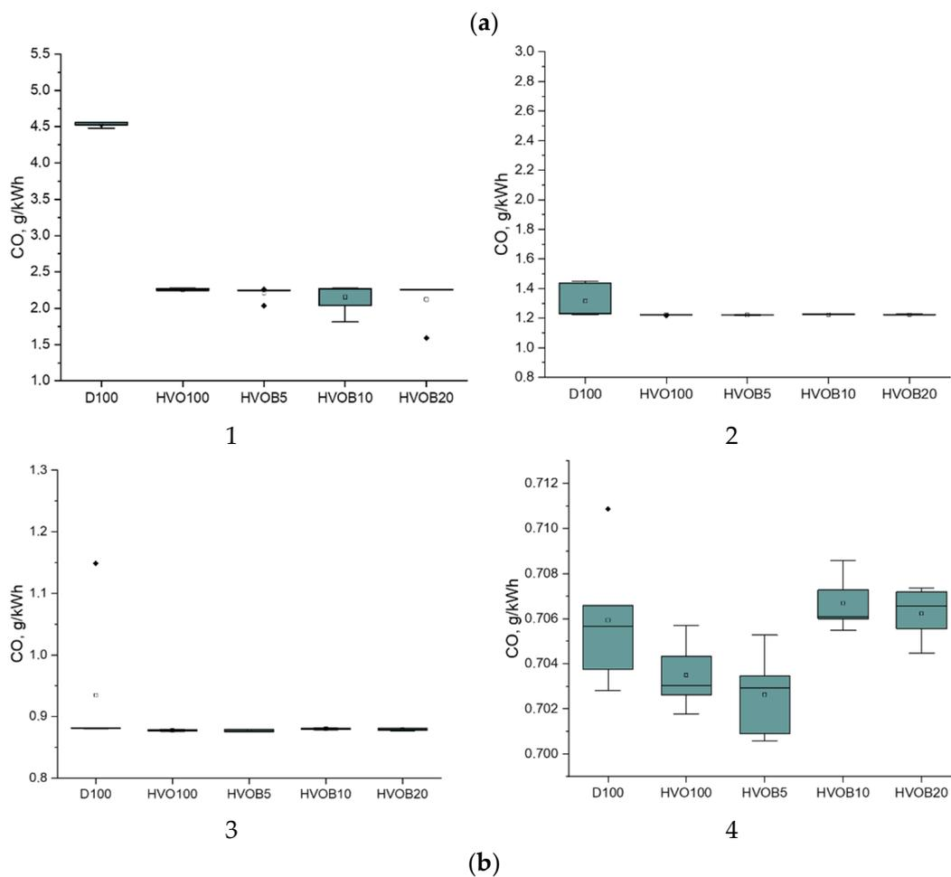
Figure 15. Dependence of CO emissions on fuel composition and engine load: (a) summary of results; (b) accuracy and errors of measurements.
