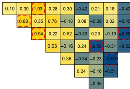
**Figure 19.** In-out tilt in assembly-wise radial power distribution with default TCP<sub>0</sub> scattering in HZ1 case.
