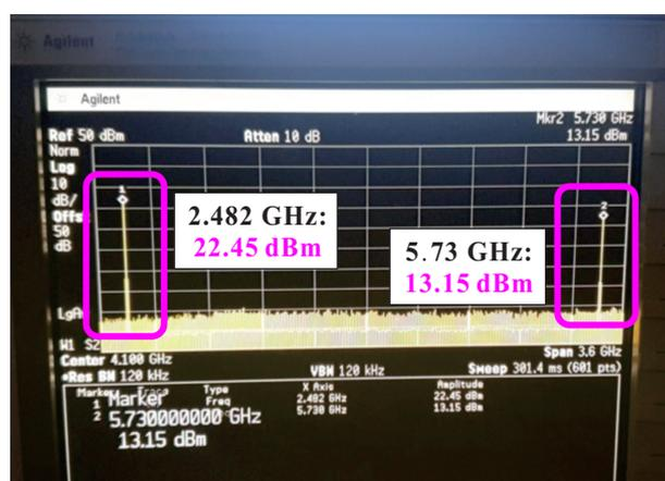
Figure 19. Screen of the spectrum analyzer when transmitting 2.482 and 5.73 GHz RF power to a dual-band Rx antenna.
