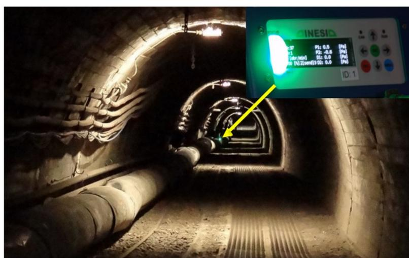
**Figure 16.** Response of the measuring module for the connector sealing (green, flashing light).
