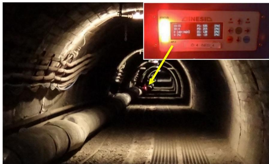
**Figure 15.** Response of the measuring module for the connector unsealing (red light).
