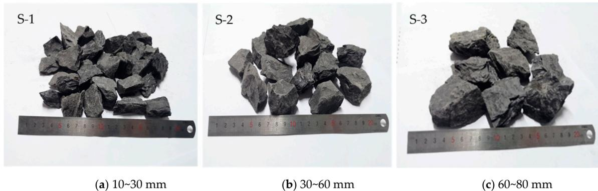
**Figure 4.** Crushed mudstone samples for the tests.
