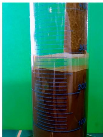
**Figure 1.** Free water in highly fractionating cement slurry.
