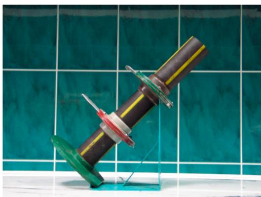
**Figure 2.** The column for testing the cement slurry fractionation.
