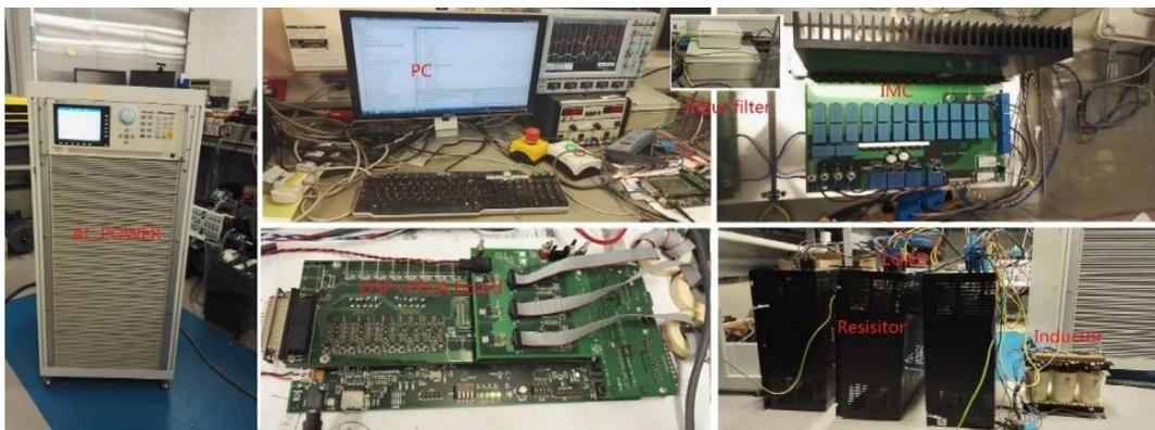
**Figure 11.** Laboratory TSMC system prototype for evaluation of the proposed control strategy.
