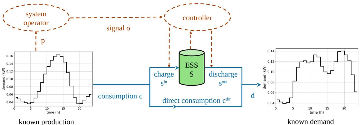
**Figure 1.** Energy system model: the power transfers between electric utility, ESS and household demand are indicated as solid lines. The dashed lines indicate signal communication (the signal which the electric utility sends to the household and the controller signals).
