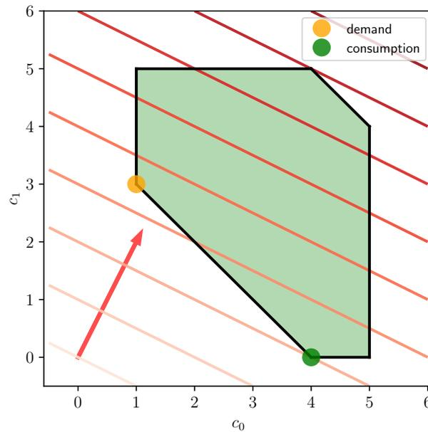
**Figure 2.** RTP in a simplified flexibility region (shaded region). The arrow depicts the price vector  $\pi$ . The contour lines of the cost function are orthogonal to the price vector. The resulting optimal consumption (dark dot) always lies at the boundary of the flexibility region.
