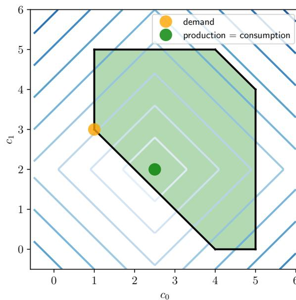
**Figure 3.** OPT in a simplified flexibility region (shaded region). The dark dot depicts the production signal to be tracked. The contour lines of the objective function are lines of constant L1-distance to the production signal. As the latter lies within the flexibility region, it coincides with the consumption profile returned by the OPT problem.
