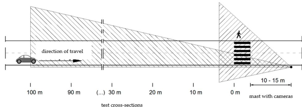
**Figure 2.** Diagram of field tests using video recording instruments.
