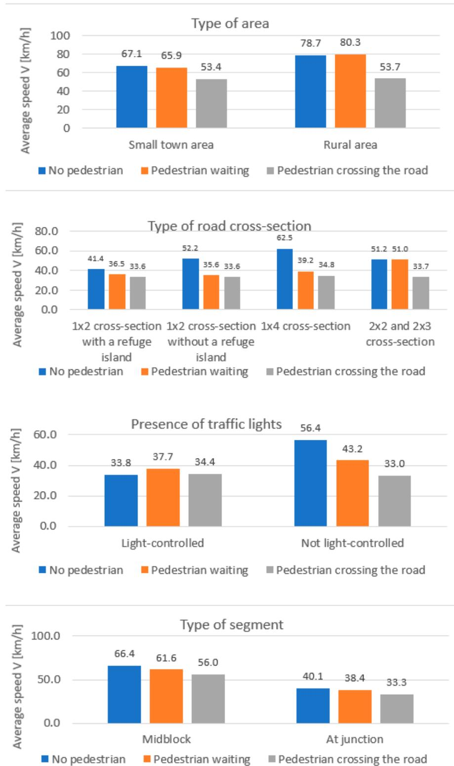
**Figure 5.** Comparison of speeds at pedestrian crossings in selected locations—speed limit of 50 km/h (measured at 50 m from the crossing).
