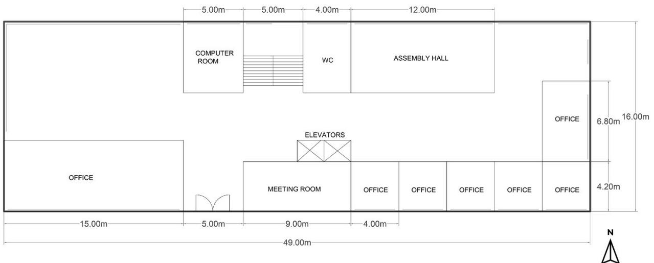
Figure 9. Plan view of the building's ground floor.
