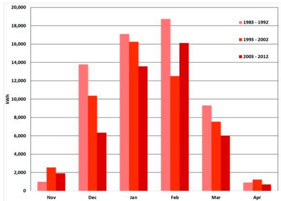
Figure 11. Total (sensible and latent) monthly energy requirements for heating.
