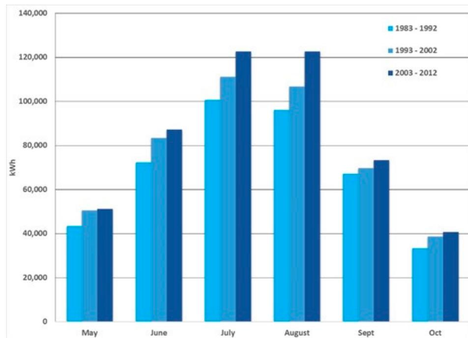
Figure 10. Total (sensible and latent) monthly energy requirements for cooling.
