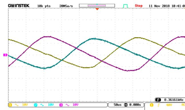
Figure 27. Three-phase AC output voltages.
