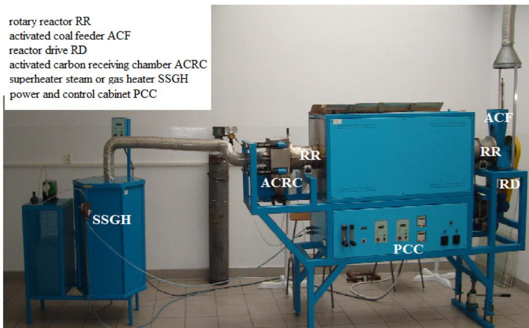
**Figure 2.** Testing stand for the high-temperature modification of activated carbon.
