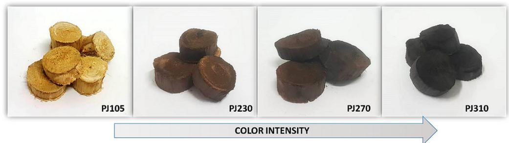
**Figure 2.** Biomass of *P. juliflora* before and after torrefaction.
