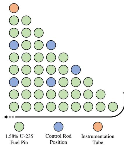
**Figure 1.** Radial pin layout of AP1000<sup>®</sup> Region B Lattice.
