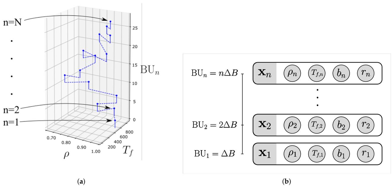
**Figure 2.** Structure of burnup sequences. (a) depiction of coolant temperature and fuel temperature change over burnup for a single burnup sequence sample; (b) structure of state vectors and evolution through burnup. Each component of  $\vec{x}$  is independently sampled from their respective distributions.
