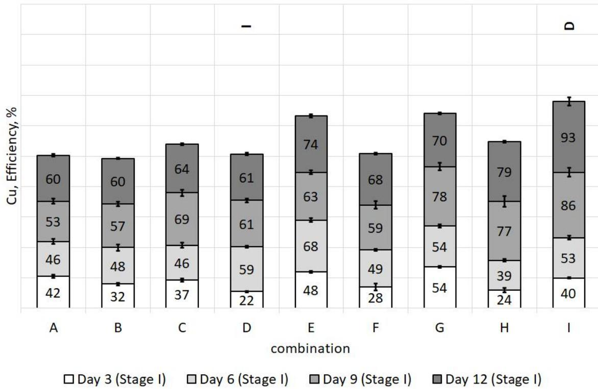
Figure 11. Effectiveness of Cu release to the dissolved fraction of leachate (Stage I).
