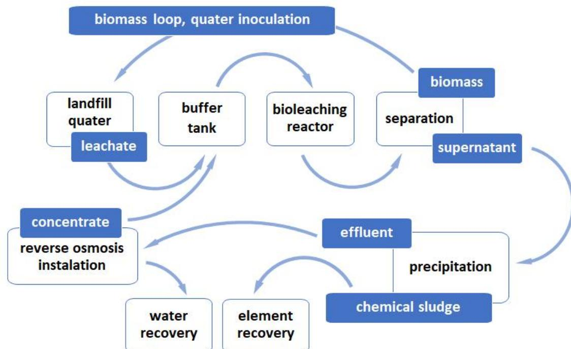
Figure 22. Scheme of an integrated solution for the treatment of landfill leachate.
