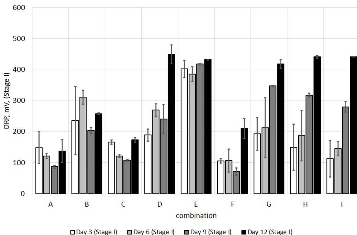
Figure 3. The oxidation and reduction potential of the samples analyzed in Stage I.
