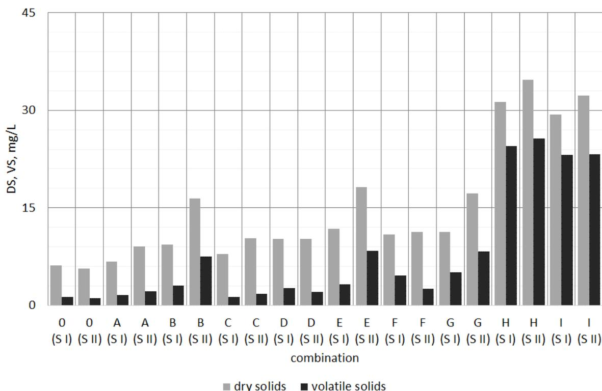
Figure 21. Dry solids and volatile solids in samples after 12 days of the process.
