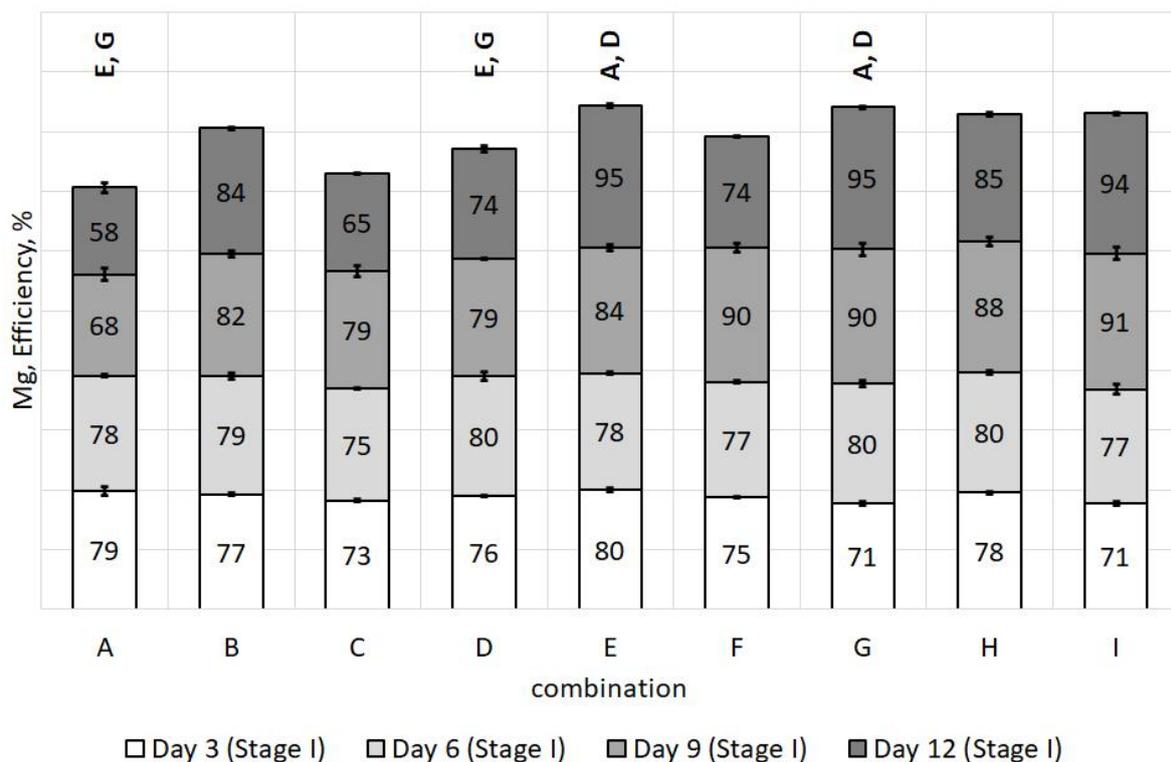
**Figure 15.** Effectiveness of Mg release to the dissolved fraction of leachate (Stage I).
