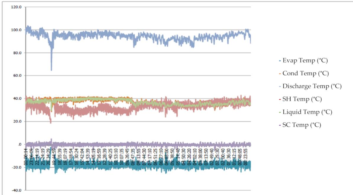
Figure 10. Temperature result for the fixed-speed semi-hermetic compressor.
