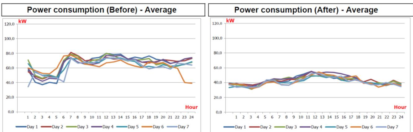
Figure 9. Average power consumption per hour before and after retrofits for store No.2 (R404A).
