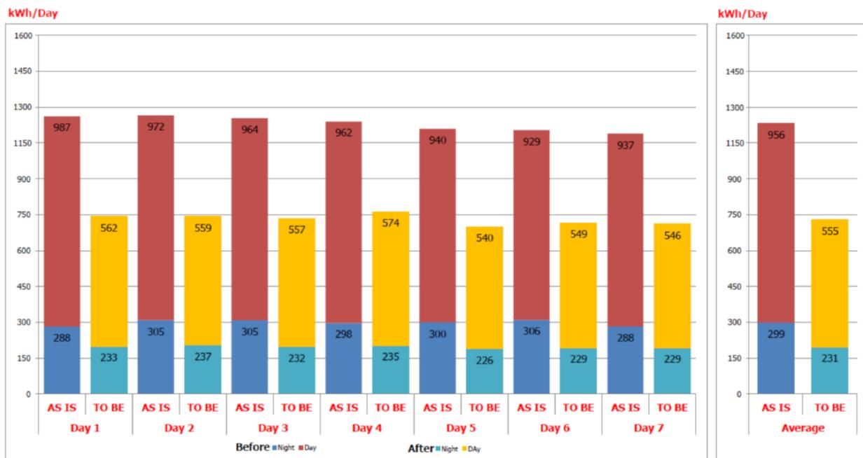
Figure 7. Average power consumption per day before and after door retrofits for store No.2 (R404A).
