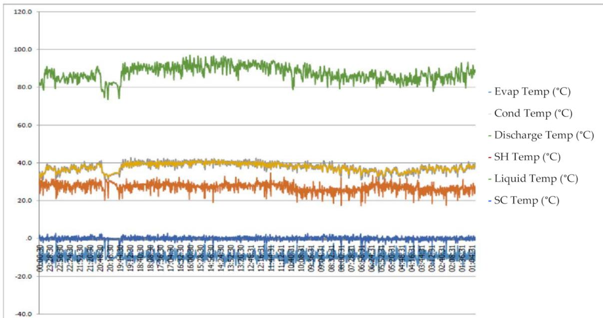
Figure 11. Temperature result for the digital-speed semi-hermetic compressor.
