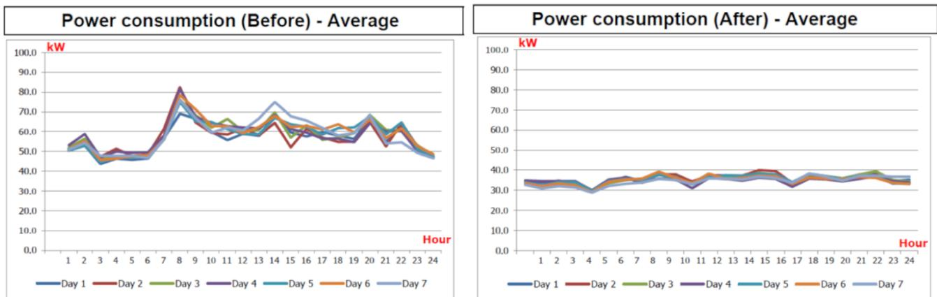
Figure 8. Average power consumption per hour before and after retrofits for store No.1 (R22).
