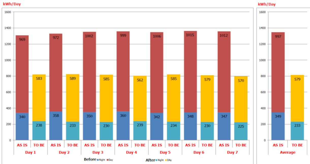
Figure 6. Average power consumption per day before and after door retrofits for store No.1 (R22).
