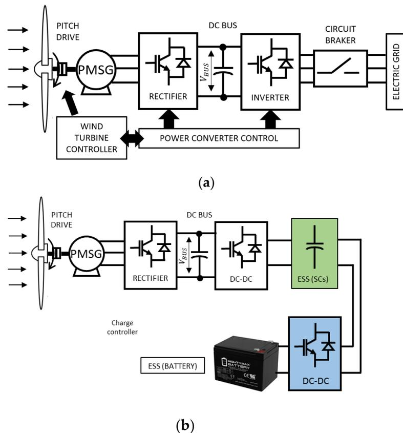
**Figure 14.** (a) Simplified electrical diagram of a variable speed wind turbine with full-scale power converter; (b) Wind Energy Conversion System with proposed HESS adapted from [60].
