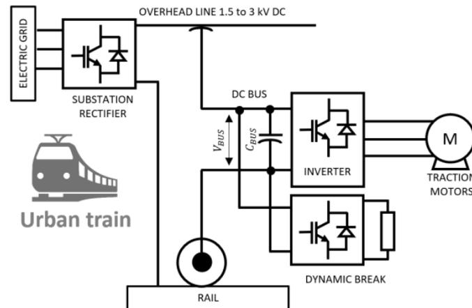
**Figure 9.** Simplified electrical diagram of the traction drive of light-rail-supplied vehicles.
