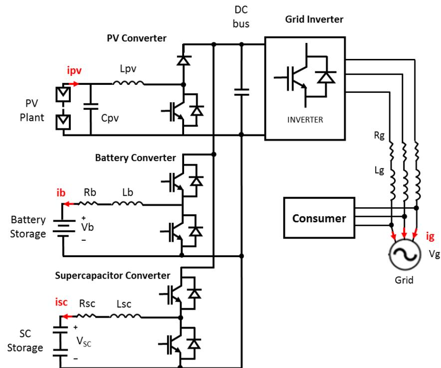
Figure 18. Scheme of model studied adapted from [78].
