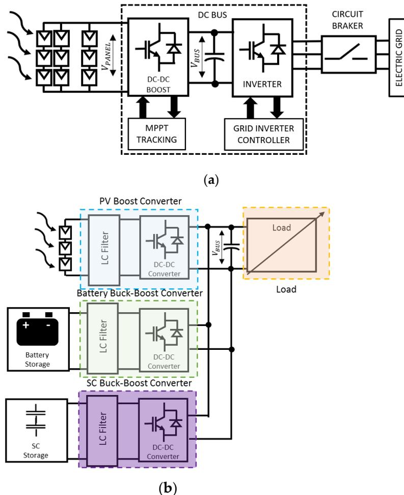
**Figure 15.** (a) Simplified electrical diagram of grid connected double conversion PV system; (b) Structure of a multiple converters configuration with maximum power point tracking (MPPT) adapted from [62].
