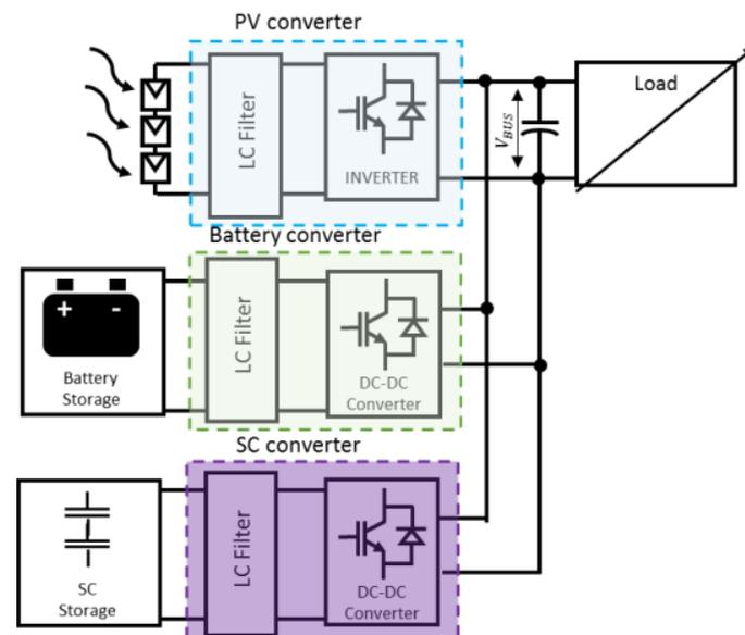
Figure 19. Scheme of the SC nanogrid adapted from [79].
