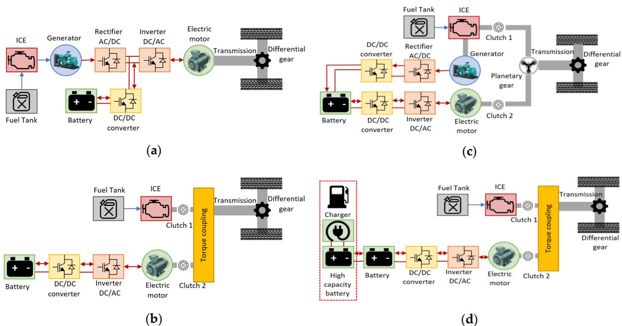
**Figure 11.** Simplified electrical diagrams of different traction drive configurations in HEV adapted from [44]: (a) ICE-based series; (b) ICE-based parallel; (c) ICE-based series-parallel; (d) ICE-based plug-in.
