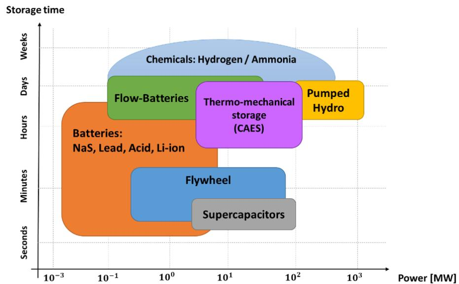
**Figure 1.** Storage time against the power delivered for electrical energy storage technologies, adapted from [5].
