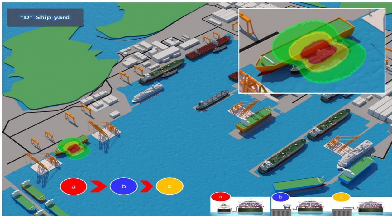
**Figure 5.** LNG bunkering arrangement diagram in shipyard “D” considering the priority of LNG bunkering method.
