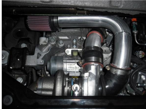
Figure 6. The turbocharged W451, 998 cc, 62 kW engine.
