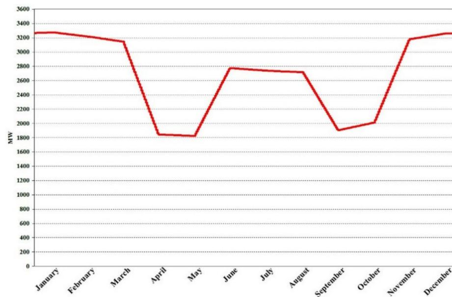
**Figure 1.** Variation of the minimum admissible generation in the EPS of Bulgaria in hourly resolution during the year 2019.
