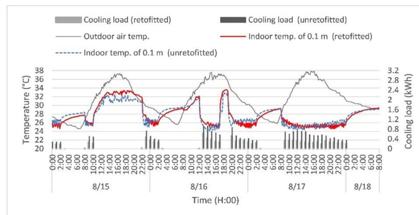
**Figure 15.** Comparison of indoor temperature and hourly cooling load at 0.1 m.
