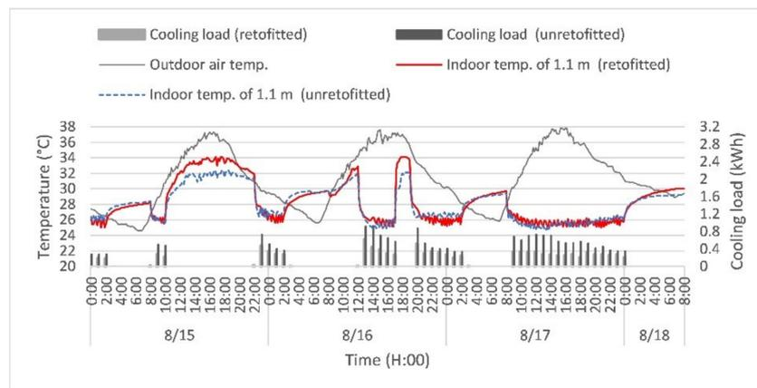
Figure 16. Comparison of indoor temperature and hourly cooling load at 1.1 m.
