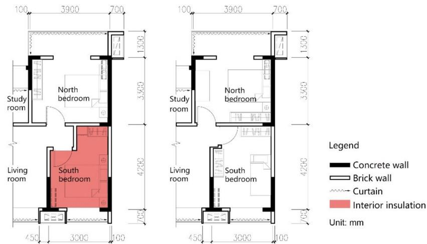
Figure 6. Layout plan of the renovation area, renovated unit (left), and original unit (right).
