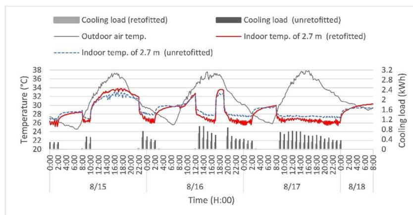
Figure 17. Comparison of indoor temperature and hourly cooling load at 2.7 m.
