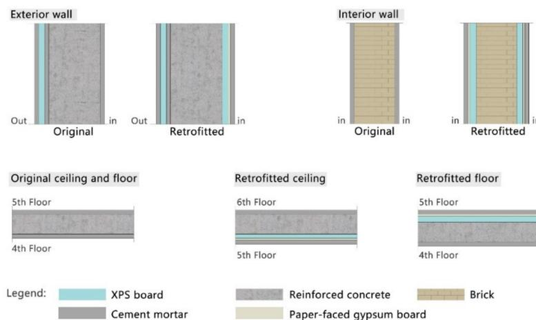
Figure 8. Configuration of the building envelope.
