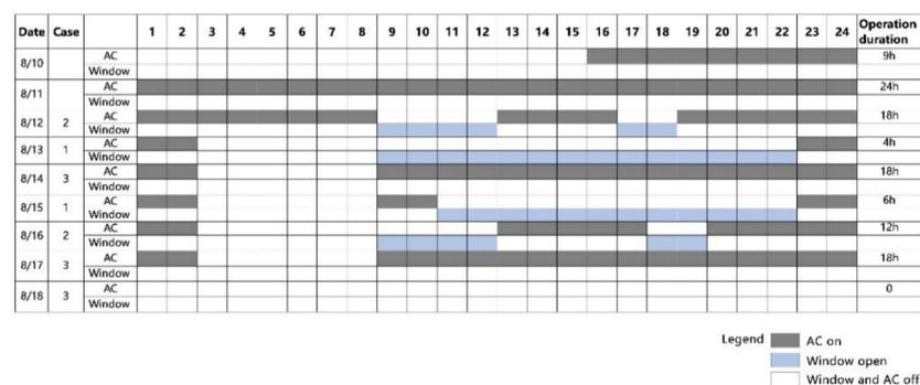
**Figure 11.** The operation schedule of the air conditioner and window.
