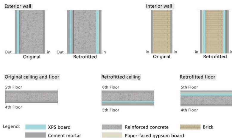
Figure 8. Configuration of the building envelope.
