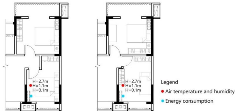
**Figure 9.** Layout of the measuring instruments, renovated unit (left), and original unit (right).
