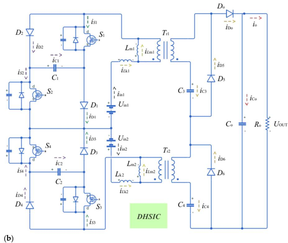
**(b)** Figure 5. New topologies of Isolated DC/DC Converter. (a) Hybrid ZVS (Zero Voltage Switching) Bidirectional DC-DC Converter; (b) Dual-Input High Step-Up Isolated Converter (DHSIC).
