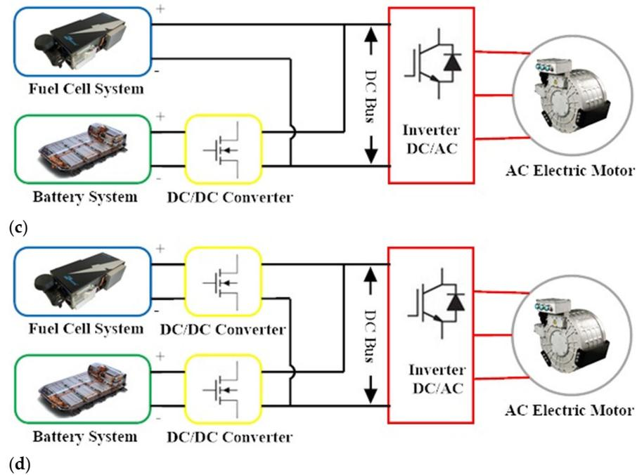
**Figure 1.** Topology of Fuel Cell Electric Vehicles (FCEVs): fuel cell + battery. (a) Topology T1; (b) Topology T2; (c) Topology T3; (d) Topology T4.
