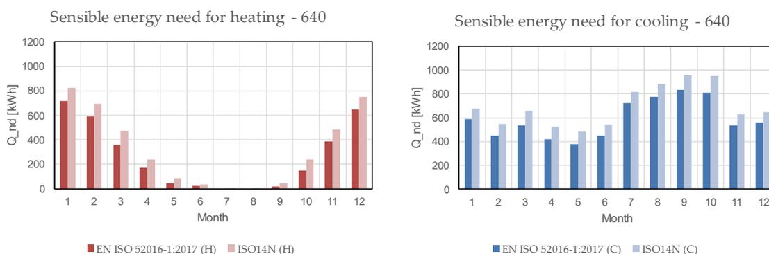
**Figure S15.** Monthly sensible energy needs for heating (solid lines) and cooling (dashed lines) for case 640 (lightweight building, intermittent thermostat control with night-time set-back for heating).
