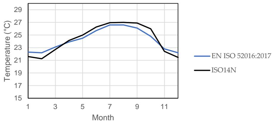
**Figure S6.** Average monthly operative temperature for case 900 (heavyweight building, continuous thermostat control strategy).
