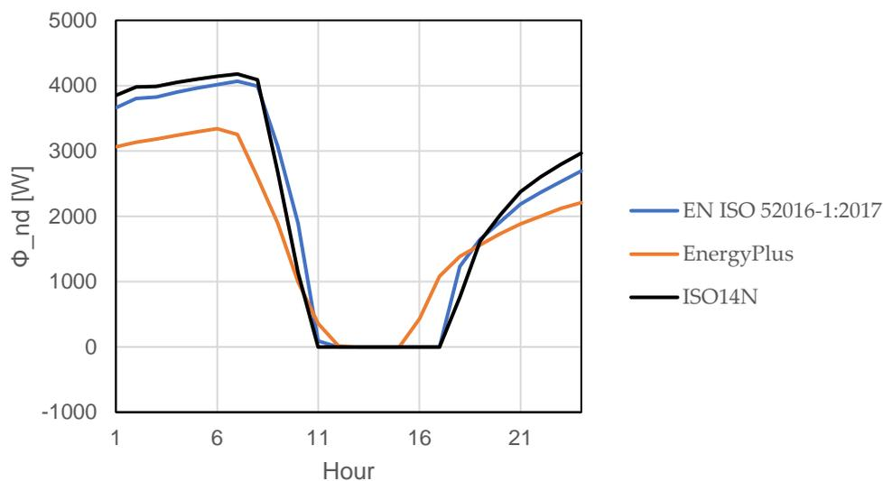
**Figure S10.** Hourly sensible heating (+) and cooling (-) load on January the 4<sup>th</sup> for case 900 (heavyweight building, continuous thermostat control strategy).
