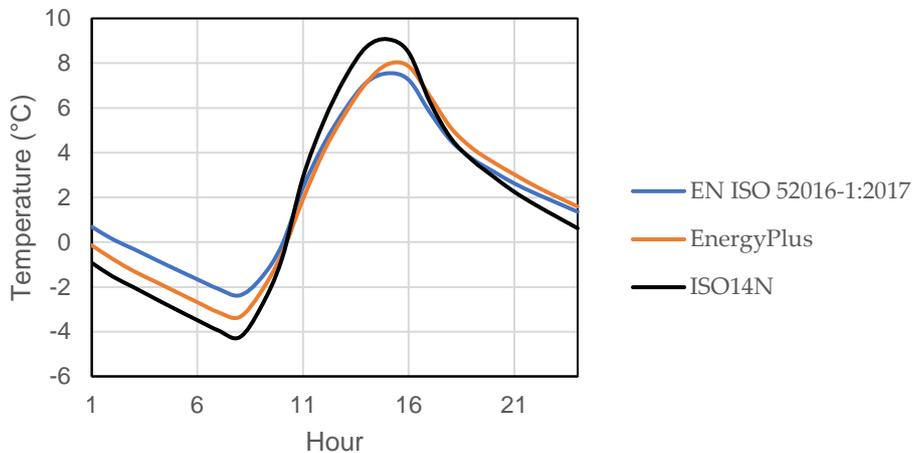
**Figure S2.** Hourly operative temperature on January the 4<sup>th</sup> for case 900FF (heavyweight building, free floating simulation).
