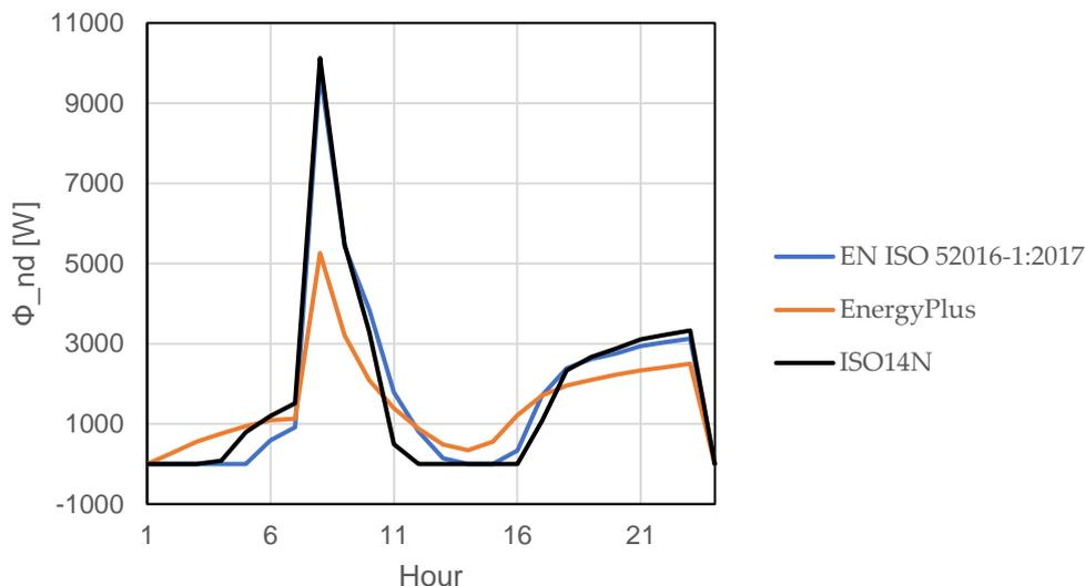
**Figure S12.** Hourly sensible heating (+) and cooling (-) load on January the 4<sup>th</sup> for case 940 (heavyweight building, intermittent thermostat control strategy with night-time set-back for heating).
