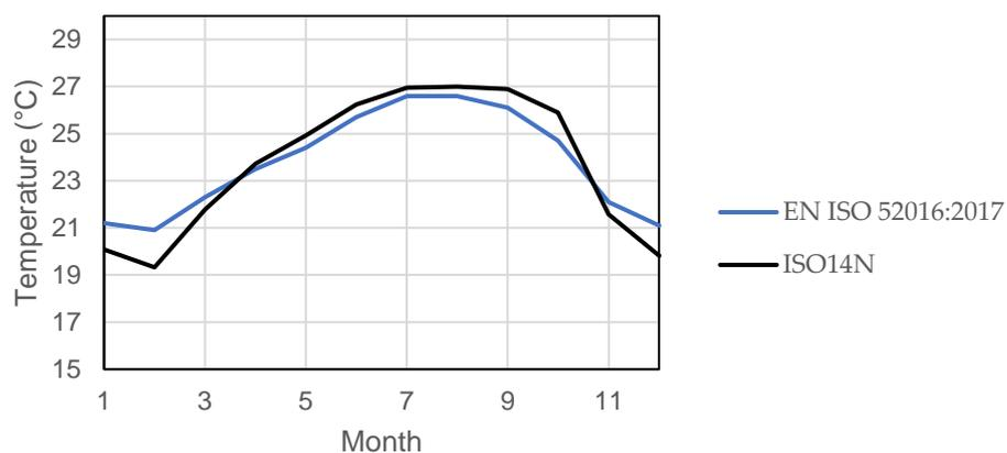
**Figure S8.** Average monthly operative temperature for case 940 (heavyweight building, intermittent thermostat control strategy with night-time set-back for heating).
