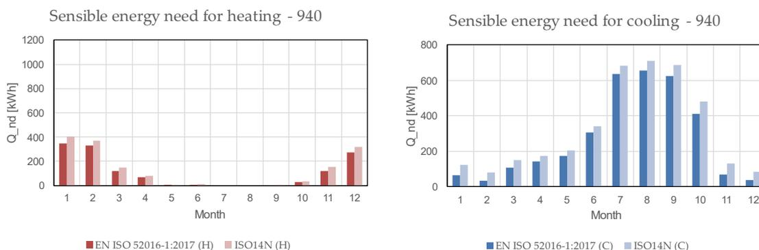
**Figure S16.** Monthly sensible energy needs for heating (solid lines) and cooling (dashed lines) for case 940 (heavyweight building, intermittent thermostat control with night-time set-back for heating).
