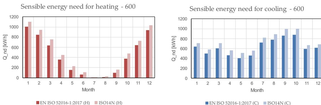
**Figure S13.** Monthly sensible energy needs for heating (solid lines) and cooling (dashed lines) for case 600 (lightweight building, continuous thermostat control strategy).
