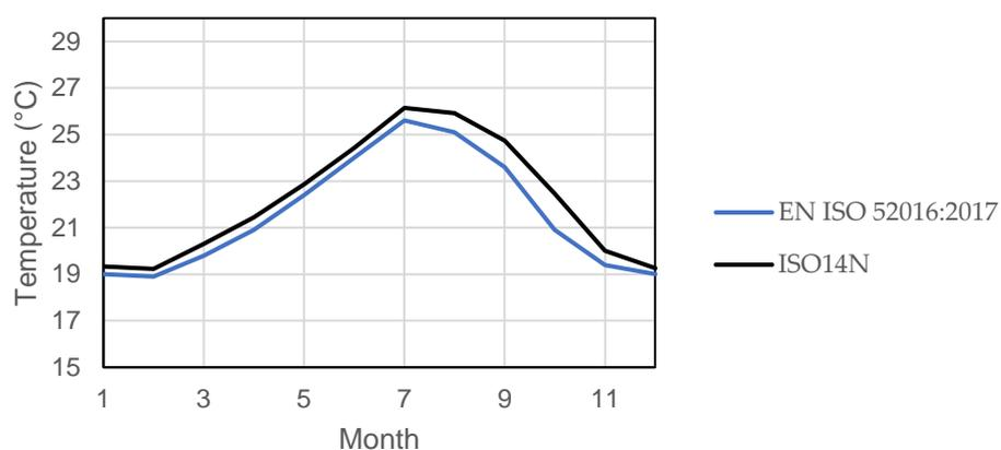
**Figure S7.** Average monthly operative temperature for case 640 (lightweight building, intermittent thermostat control strategy with night-time set-back for heating).
