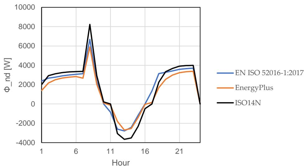
**Figure S11.** Hourly sensible heating (+) and cooling (-) load on January the 4<sup>th</sup> for case 640 (lightweight building, intermittent thermostat control strategy with night-time set-back for heating).
