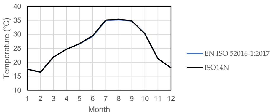
**Figure S4.** Average monthly operative temperature for case 900FF (heavyweight building, free floating simulation).
