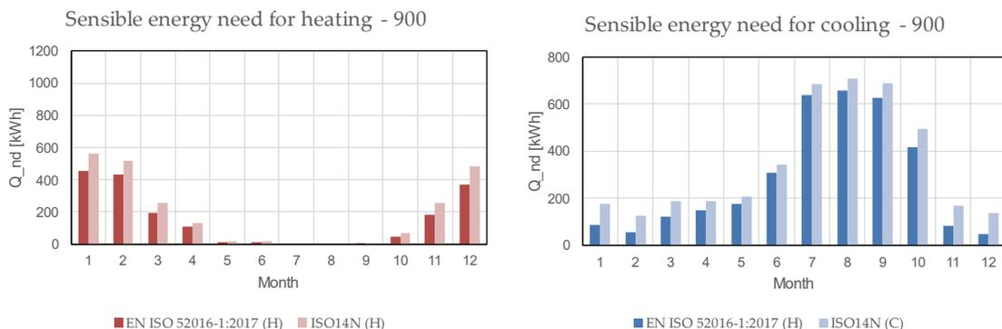
**Figure S14.** Monthly sensible energy needs for heating (solid lines) and cooling (dashed lines) for case 900 (heavyweight building, continuous thermostat control strategy).
