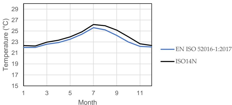
**Figure S5.** Average monthly operative temperature for case 600 (lightweight building, continuous thermostat control strategy).
