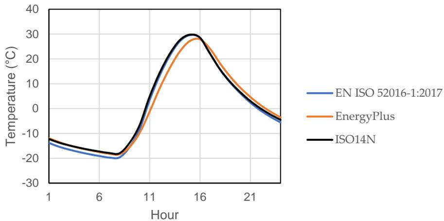
**Figure S1.** Hourly operative temperature on January the 4<sup>th</sup> for case 600FF (lightweight building, free floating simulation).
