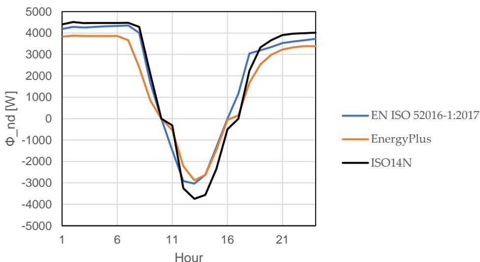
**Figure S9.** Hourly sensible heating (+) and cooling (-) load on January the 4<sup>th</sup> for case 600 (lightweight building, continuous thermostat control strategy).
