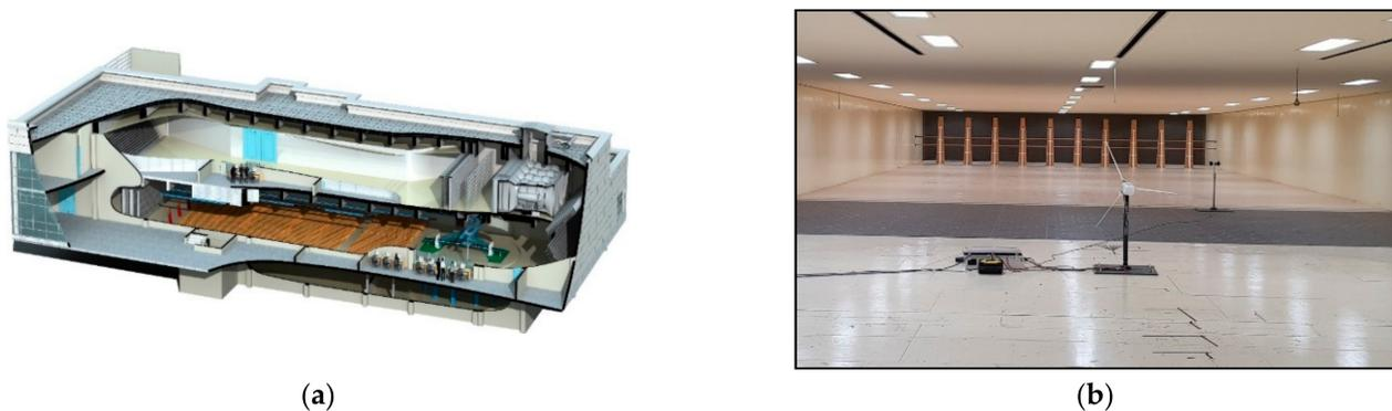
**Figure 8.** Wind tunnel test: (a) configuration of wind tunnel; (b) view of testing wind turbine.
