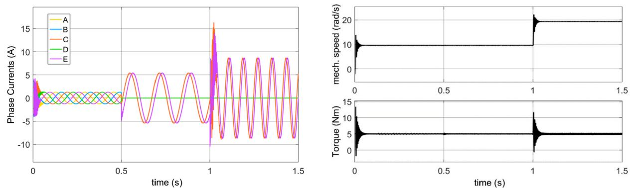
**Figure 18.** MATLAB/Simulink simulation results of the NATPOC fault-tolerant control currents.
