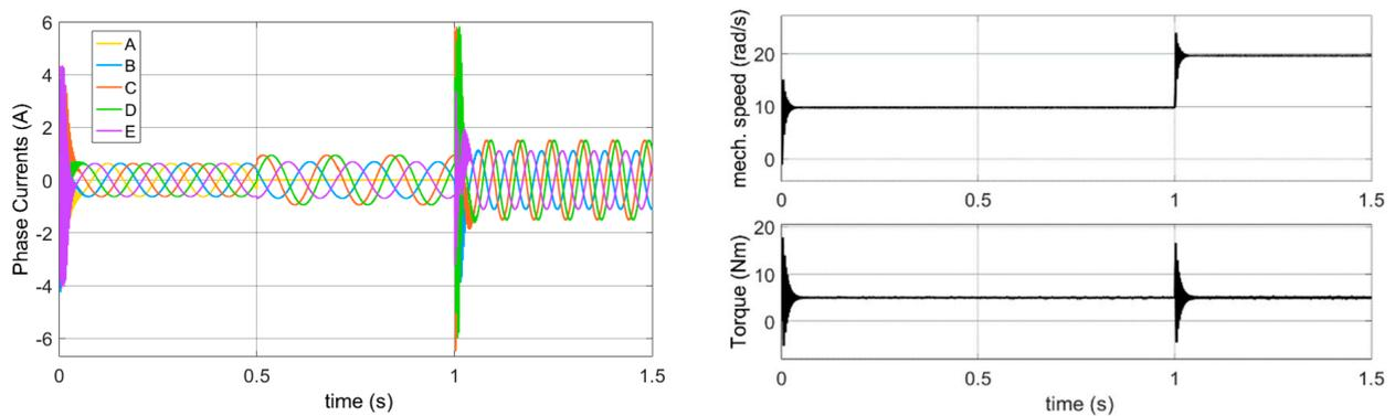
Figure 14. MATLAB/Simulink simulation results of the SPOC fault-tolerant control currents.
