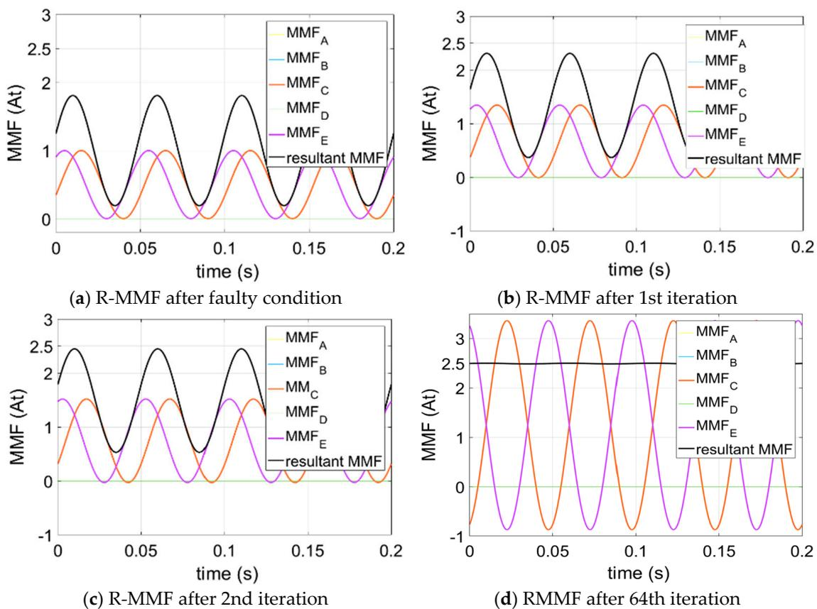
Figure 11. Non-adjacent three-phase open-circuit (NATPOC) condition resultant MMFs.
