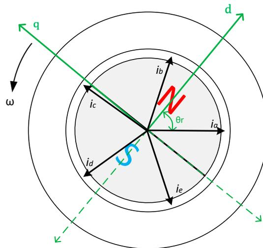
**Figure 1.** Illustration of the direct and quadrature (d-q) axes for the two-pole five-phase permanent magnet (PM) machine.
