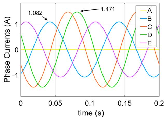
**Figure 4.** SPOC condition fault-tolerant control currents.
