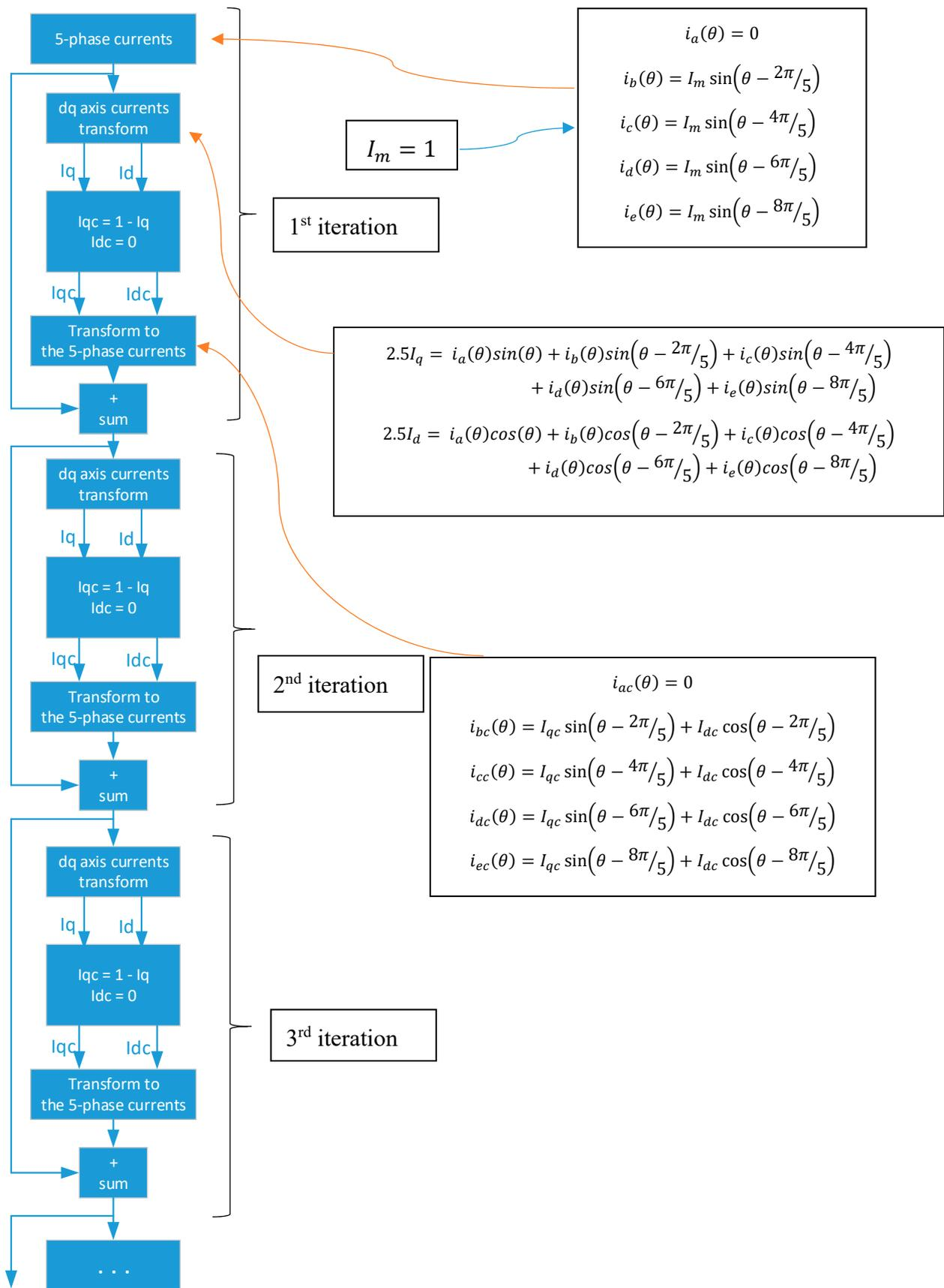
Figure 2. Flow diagram to obtain the remaining healthy phase currents.
