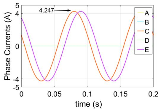
Figure 12. NATPOC condition fault-tolerant control currents.
