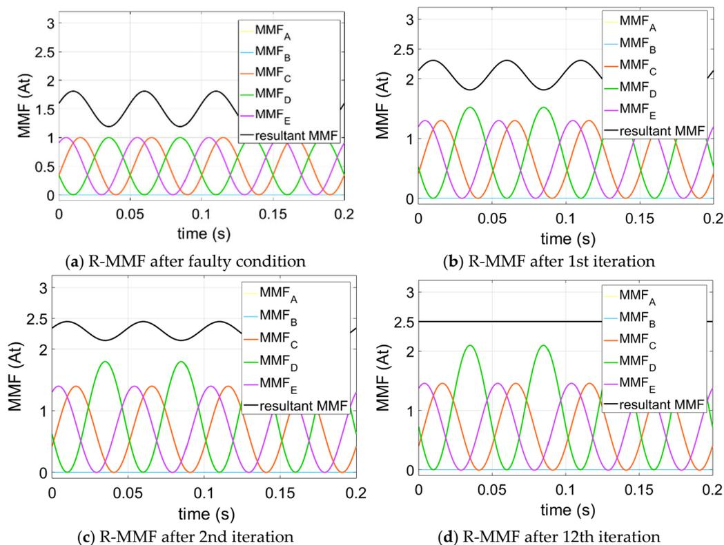
**Figure 5.** Adjacent double-phase open-circuit (ADPOC) condition resultant MMFs.
