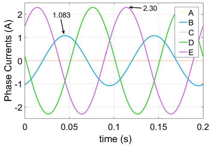
Figure 8. NADPOC condition fault-tolerant control currents.
