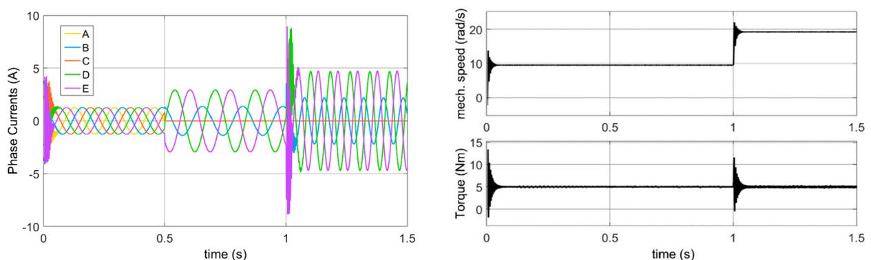
Figure 16. MATLAB/Simulink simulation results of the NADPOC fault-tolerant control currents.
