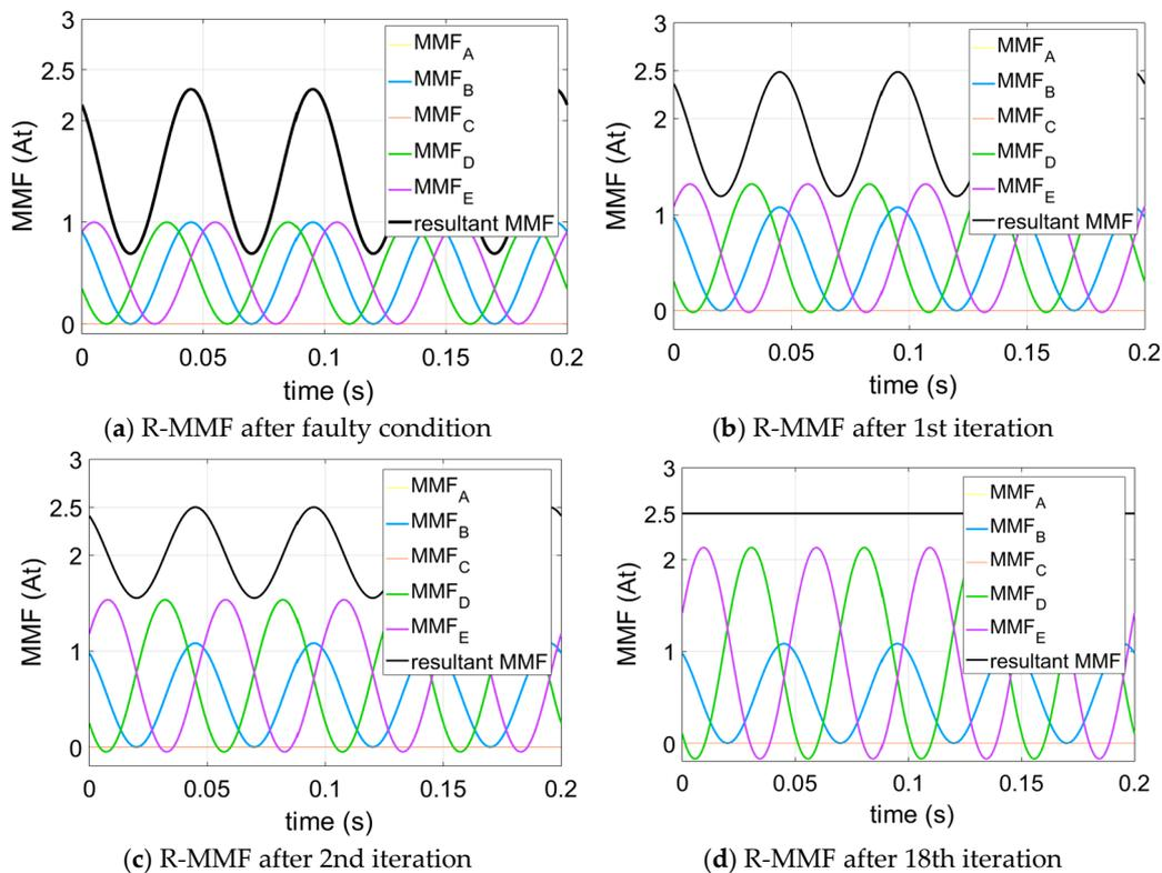
Figure 7. Non-adjacent double-phase open-circuit (NADPOC) condition resultant MMFs.
