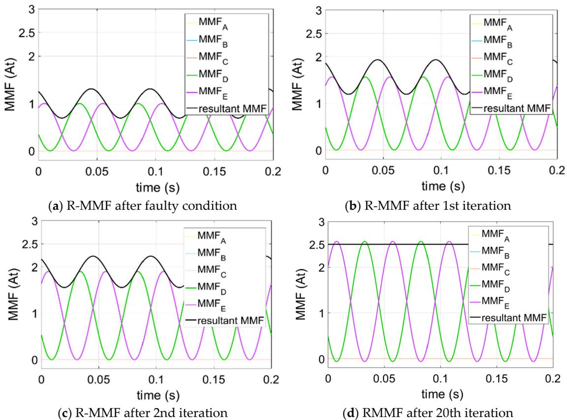
Figure 9. Adjacent three-phase open-circuit (ATPOC) condition resultant MMFs.
