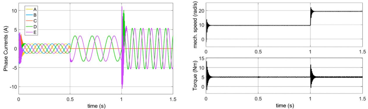
**Figure 17.** MATLAB/Simulink simulation results of the ATPOC fault-tolerant control currents.
