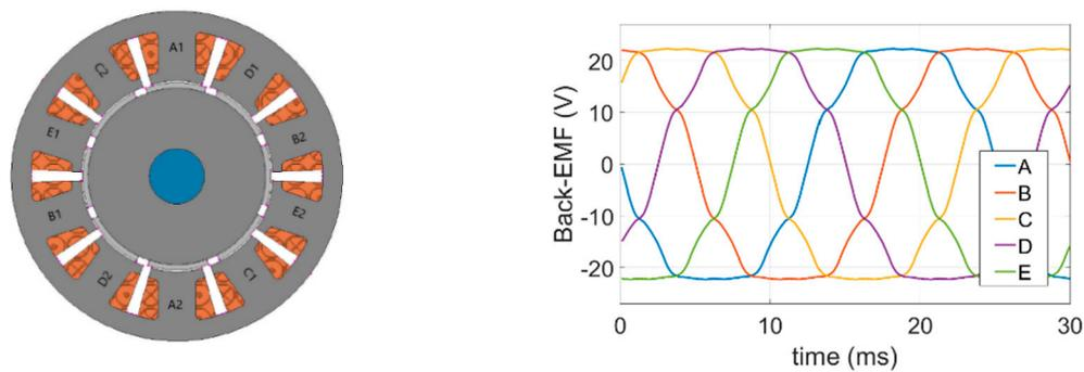
**Figure 19.** Modelled Five-phase PM machine and its back-EMF waveform.
