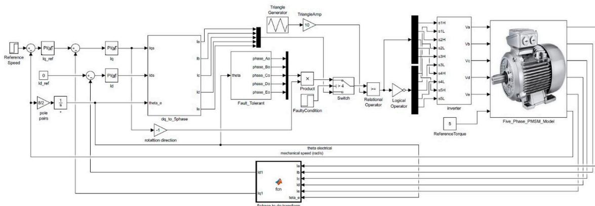
Figure 13. MATLAB/Simulink block diagram of the open-circuit fault-tolerant control.
