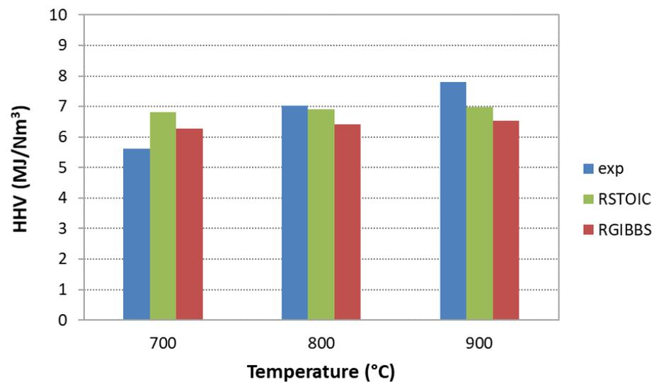
Figure S6. Effect of the variation of HHV with temperature for the gasification of PKS with SR = 0.2 and 70 vol.% steam.
