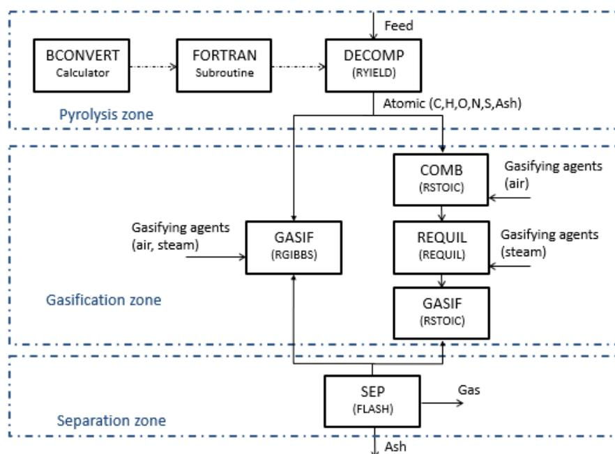
Figure S1. Flow chart of the simulation procedure for the steam gasification process.
