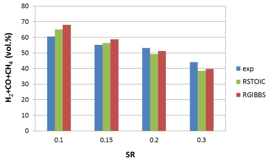
**Figure S2.** Comparison between experiment and simulation data of combustible gas concentration at different stoichiometric ratios, for the gasification of PKS with 70 vol.% steam at 900 °C.
