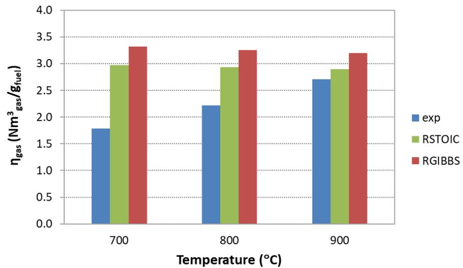
**Figure S5.** Effect of the variation of  $\eta_{gas}$  with temperature for the gasification of PKS with SR = 0.2 and 70 vol.% steam.
