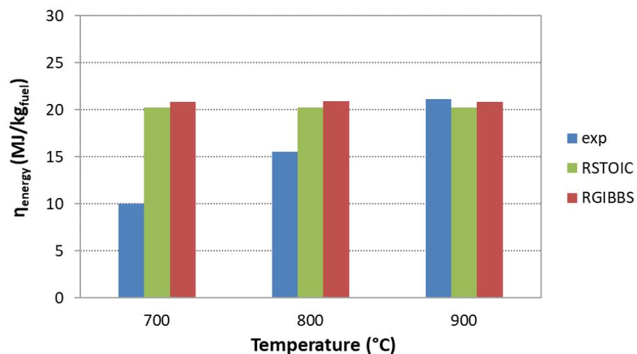
Figure S7. Effect of the variation of temperature on  $\eta_{\text{energy}}$  for the gasification of PKS with SR = 0.2 and 70 vol.% steam.
