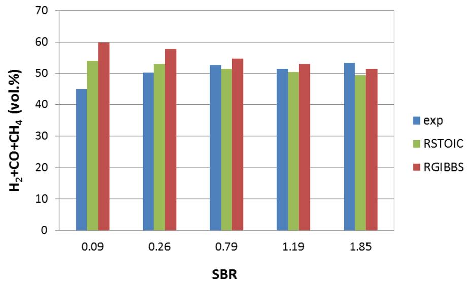
**Figure S3.** Comparison between experiment and simulation data of combustible gas concentration at different steam to biomass ratios, for the gasification of PKS at 900 °C with SR = 0.2.
