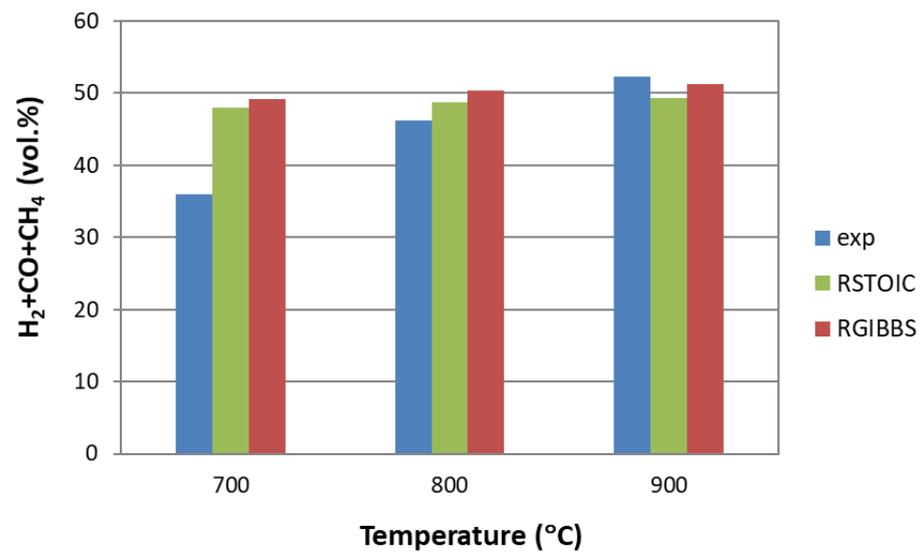
**Figure S4.** Comparison between experiment and simulation data of combustible gas concentration at different temperatures, for the gasification of PKS at SR = 0.2 and 70 vol.% steam.
