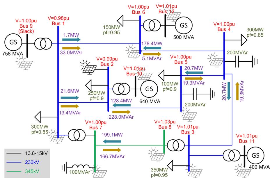
**Figure 2.** Single line diagram for the modified benchmark network with PV plant connected to bus 2 and values corresponding to approximately 65% (1450 MW) load level. The transmission circuit was completely assessed for PV connection at any of its buses.
