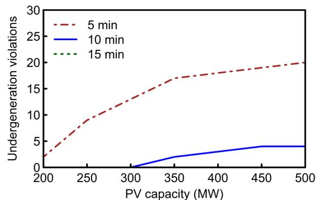
**Figure 8.** Under-generation violation count at increasing PV penetration rate. Under-generation occurs when PV becomes suddenly shaded and thermal units cannot ramp up fast enough to supply deficit power.
