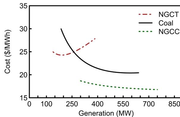
**Figure 4.** The operation cost in \$/MWh including the fuel and auxiliary costs for the thermal units considered. The cost rate in \$/h can be calculated as a product of the operation cost and the generation.
