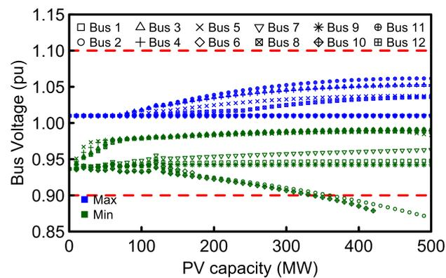
**Figure 13.** The maximum and minimum bus voltage variation for increasing PV capacity over multiple points of interconnection (POI). A PV capacity is undesirable if it leads to bus voltage variation above 1.1 or below 0.9 pu.
