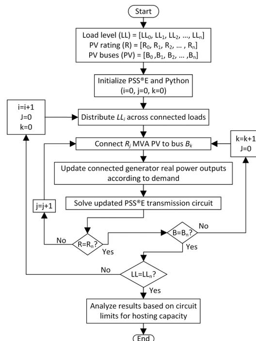
**Figure 12.** Operational flow chart for the proposed framework for estimating the hosting capacity on a transmission network. The steady-state impact for increasing solar PV capacity at different POI was evaluated to estimate the maximum PV hosting capacity for the network.
