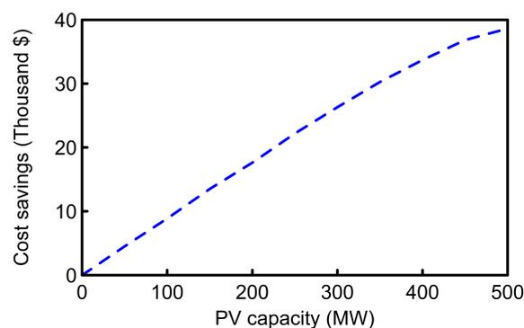
**Figure 11.** Operation cost saving due to increase in PV penetration. For the example day considered, an increase in operation cost was observed for PV penetrations below 500 MW due to operation of inefficient units to meet demand.
