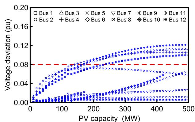
**Figure 14.** Maximum bus voltage deviation for defined PV capacity. A violation is recorded if the maximum voltage deviation exceeds 0.08 pu. The maximum voltage deviation is also an indicator of the expected voltage variation due PV intermittency.
