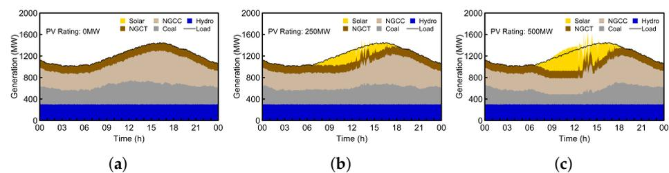
**Figure 6.** Minute-to-minute (M-M) unit economic dispatch highlighting the impact of increasing PV penetration on an example generation portfolio. The results indicate that large PV penetrations may lead to both over- and under-generation scenarios where combined power from units cannot match demand. The presented analysis include (a) no PV, (b) 250 MW PV, and (c) 500 MW PV penetration case studies.
