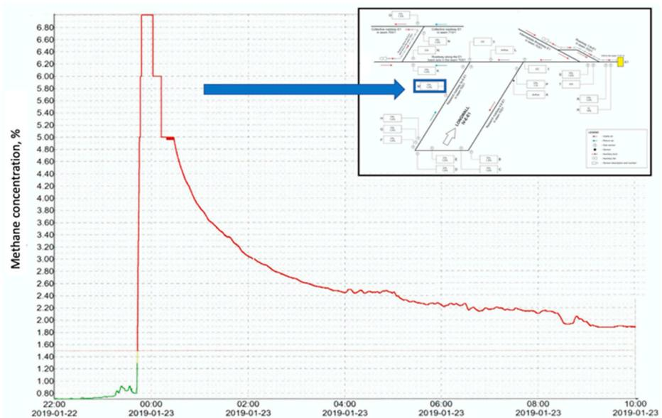
**Figure 11.** A change in methane concentration after the burst recorded by a CH<sub>4</sub> (M) sensor installed in Researcher roadway 3a-E-E1 in seam 703/1 5 m ahead of a transformer (sensor M in Figure 4) [3].
