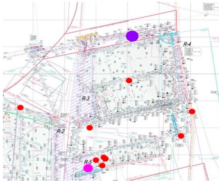
**Figure 6.** The map of seam 409/3 in the area of longwall H-4 with indicated spots where bumps occurred with an energy of  $10^6$ – $10^8$  J.
